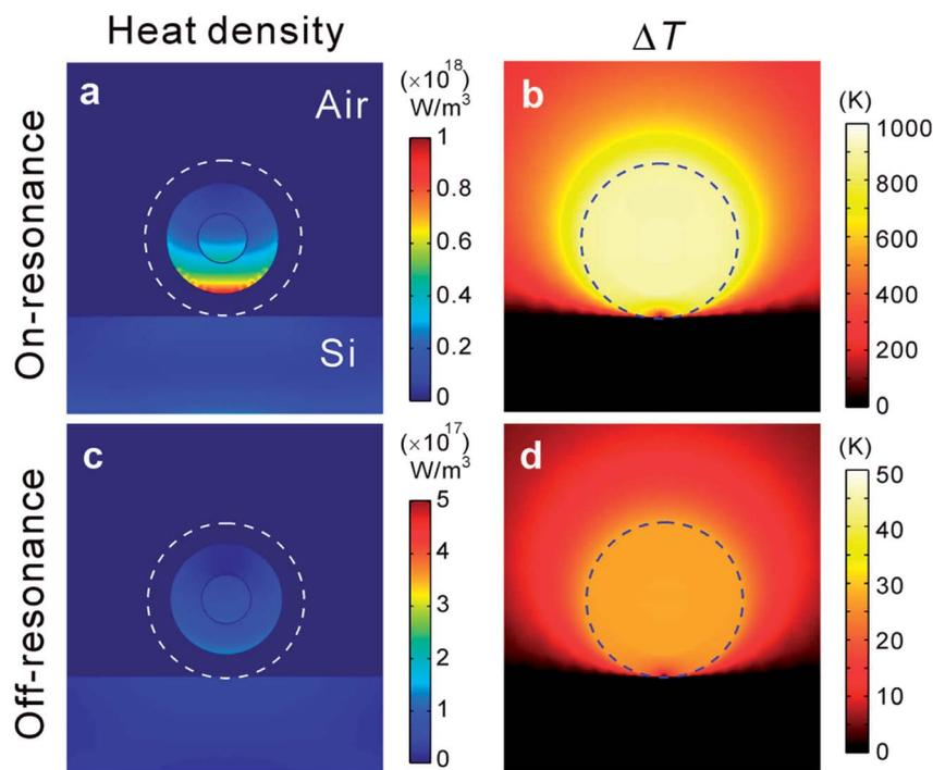
Fig. 4 Numerical calculations of plasmonic heating by laser irradiation. (a and c) Heat source density distribution and (b and d) increased temperature ( $\Delta T$ ) of a GERT on the Si substrate under on-resonant (532 nm) or off-resonant (785 nm) excitation with a power density of  $3 \times 10^5\text{ W cm}^{-2}$ . Dashed circles indicate the diameter of the GERT.
