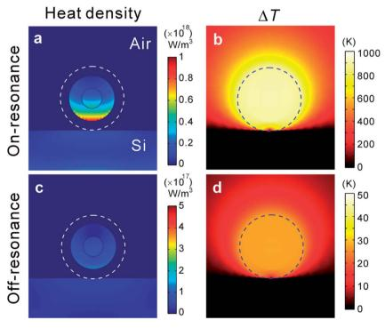
Fig. 4 Numerical calculations of plasmonic heating by laser irradiation. (a and c) Heat source density distribution and (b and d) increased temperature ( $\Delta T$ ) of a GERT on the Si substrate under on-resonant (532 nm) or off-resonant (785 nm) excitation with a power density of 3  $\times$ 10<sup>5</sup> W cm<sup>-2</sup>. Dashed circles indicate the diameter of the GERT.
