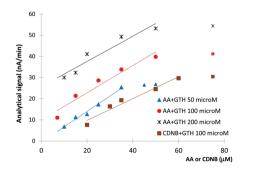
Fig. 4 The calibration curves for AA obtained with three different GSH concentrations. A comparison with CDNB is also presented using 100 μM GSH. The calibration curve is calculated using only the signals for the first 5 concentrations as a plateau is reached for higher concentrations
