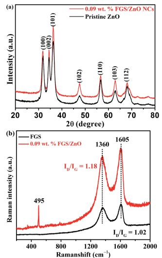
Fig. 1 (a) XRD spectra and (b) Raman spectra of pristine ZnO and FGS/ ZnO (0.09 wt%) NCs.
