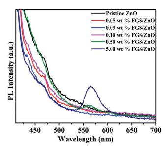
Fig. 4 The photoluminescence (PL) spectra of pristine ZnO NPs and FGS/ZnO NCs.
