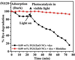
Fig. 7 (a) Determination of hydroxyl radical formation on the surface of various photocatalysts under visible light irradiation using photoluminescence spectroscopy ( $\lambda_{exc} = 315$  nm) and (b) photodegradation of safranin-T using 0.09 wt% FGS/ZnO NCs in the presence of histidine as a scavenger.
