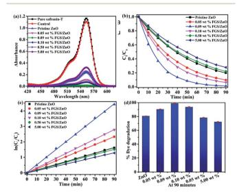
Fig. 5 (a) Photodegradation of safranin-T using pristine ZnO NPs and FGS/ZnO NCs, (b) comparison of the photocatalytic activity of FGS/ZnO NCs with that of pristine ZnO NPs, (c) plots of  $\ln(C_{\rm o}/C_{\rm c})$  vs. irradiation time using different photocatalysts and (d) comparison of safranin-T photodegradation efficiency using ZnO NPs and FGS/ZnO NCs.
