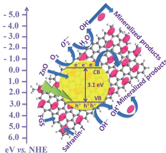
Fig. 6 Proposed photocatalytic mechanism for the degradation of safranin-T dye using FGS/ZnO NCs.<sup>24,27,29</sup>
