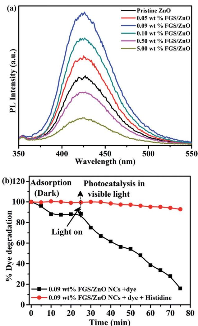
Fig. 7 (a) Determination of hydroxyl radical formation on the surface of various photocatalysts under visible light irradiation using photoluminescence spectroscopy ( $\lambda_{\text{exc}} = 315$  nm) and (b) photodegradation of safranin-T using 0.09 wt% FGS/ZnO NCs in the presence of histidine as a scavenger.
