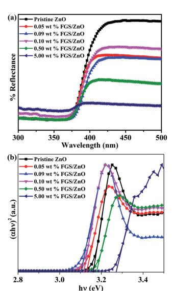
Fig. 3 (a) The UV-visible diffuse reflectance spectra and (b) Tauc plots of pristine ZnO NPs and FGS/ZnO NCs.
