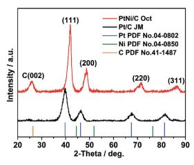
Fig. 2 XRD patterns of the octahedral PtNi/CNT catalyst and Pt/C (JM).
