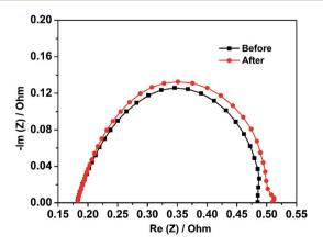
Fig. 7 The EIS results of the MEA fabricated using the octahedral PtNi/ CNT catalyst in the cathode before and after a high potential durability test.
