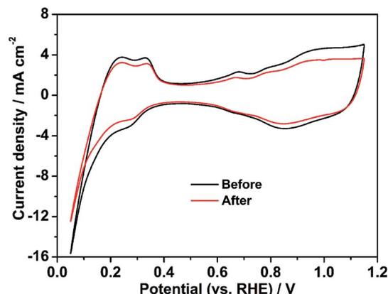
Fig. 6 The *in situ* CV curves of the MEA fabricated using the octahedral PtNi/CNT catalyst in the cathode before and after a high potential durability test.
