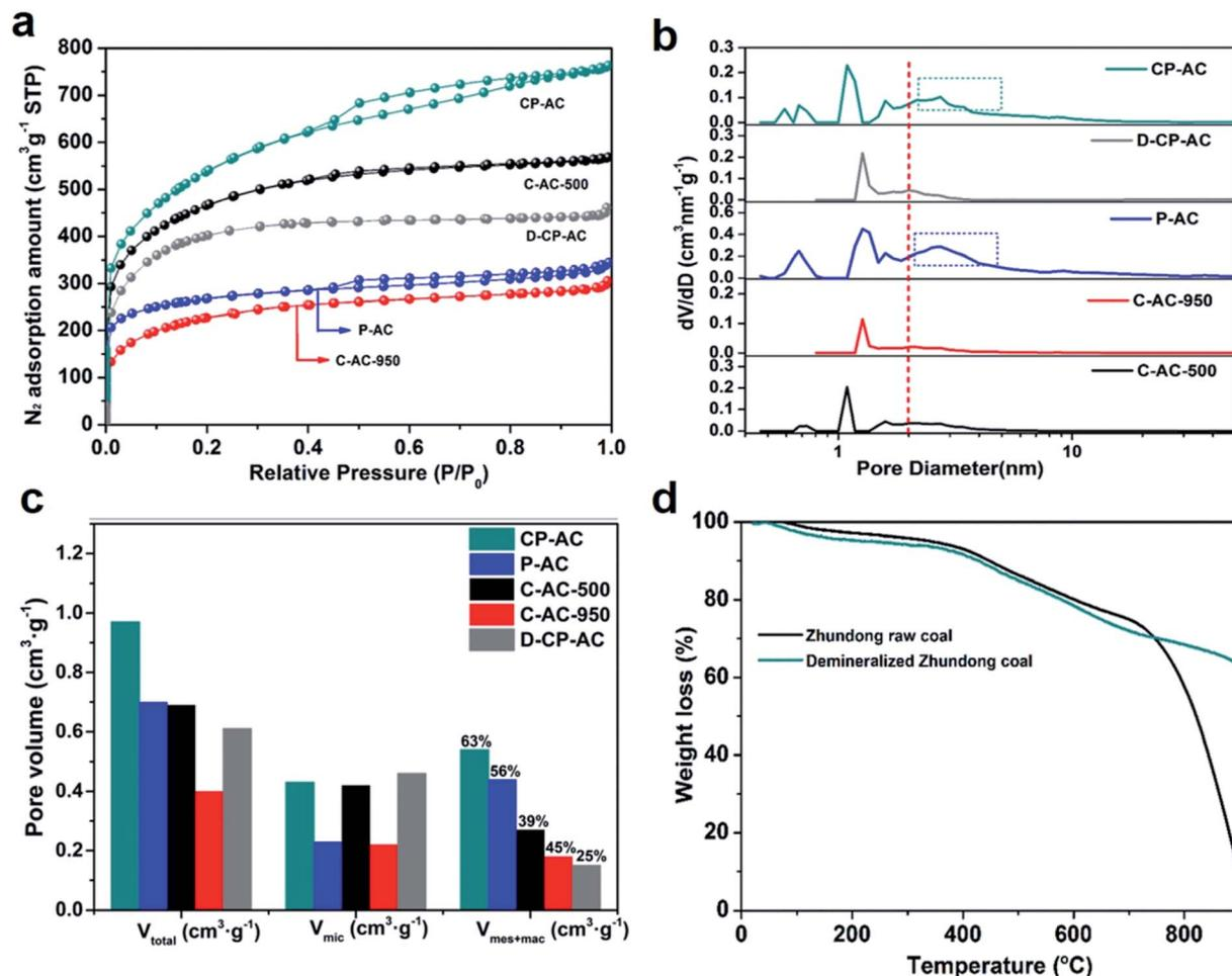
Fig. 2 (a) N<sub>2</sub> adsorption isotherms of prepared activated carbons; (b) DFT pore size distributions of prepared activated carbons; (c) pore volume distributions of prepared activated carbons with various pore size ranges; (d) TGA profiles of Zhundong raw coal and demineralized Zhundong coal under simulated CO<sub>2</sub> physical activation process.
