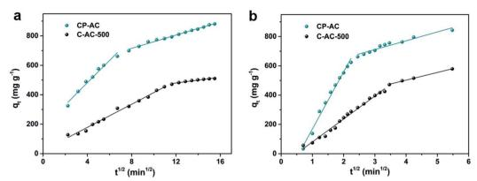
Fig. 7 RhB adsorption kinetic results of typical samples. (a) Intraparticle model fitting for saturation adsorption test; (b) intraparticle model fitting for sonication-assisted adsorption test.
