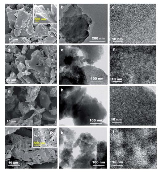
Fig. 1 SEM and TEM images of Zhundong raw coal and the derived activated carbons obtained by various activation procedures. SEM (a), TEM (b) and HRTEM (c) images of Zhundong coal; SEM (d), TEM (e) and HRTEM (f) images of CP-AC; SEM (g), TEM (h) and HRTEM (i) images of C-AC; SEM (j), TEM (k) and HRTEM (l) images of P-AC.
