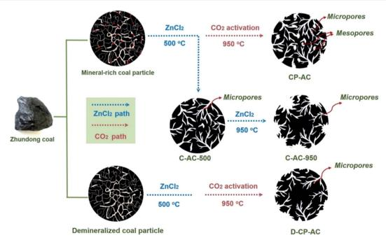
Fig. 4 A schematic illustration of the porosity development mechanism by various strategies.
