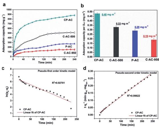
Fig. 5 RhB adsorption kinetic results of typical samples. (a) Adsorption capacities as a function of time; (b) normalized adsorption capacity to BET surface areas for typical samples; (c) pseudo-first order kinetic fitting for CP-AC; (d) pseudo-second order kinetic fitting for CP-AC.
