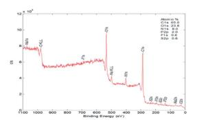
Fig. 3 XPS spectra of BODIPY-O-CMC-cRGD.
