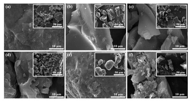
$\label{eq:Fig. 1} \textbf{Fig. 1} \quad \text{SEM images of the LS (a), LSC (b), LS-SO}_3H \ \text{(c), LSC}_{300} - \text{SO}_3H \ \text{(d), AL (e), and AL-SO}_3H \ \text{(f)}.$
