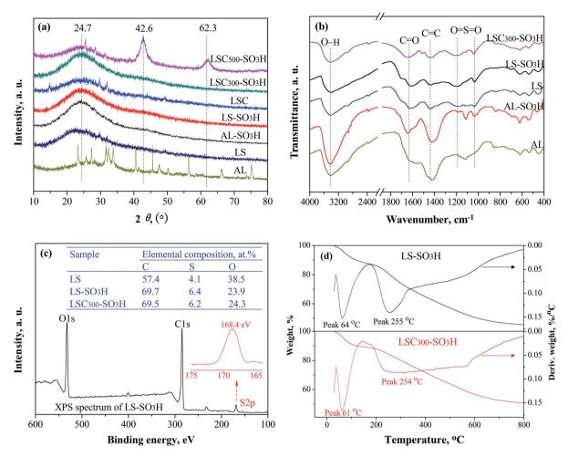
Fig. 2 XRD patterns (a), FT-IR spectra (b), XPS analyses (c), and TGA curves (d) of the samples.
