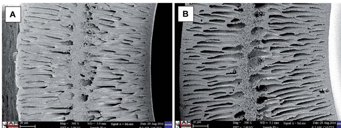
Fig. 4 Cross-section morphology of (A) the modified membrane, and (B) the reference membrane; 500× magnification.
