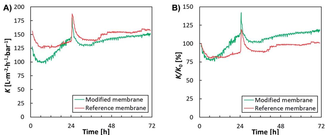
Fig. 2 Permeability over time: (A) absolute values ( $K$ ) for the modified and reference membranes, (B) normalised permeability ( $K/K_0$ ), after eliminating the influence of different feed characteristics.
