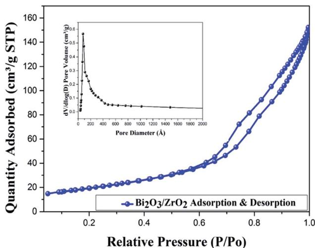
Fig. 4  $\text{N}_2$  adsorption–desorption isotherm of 2.5%  $\text{Bi}_2\text{O}_3/\text{ZrO}_2$  catalyst.
