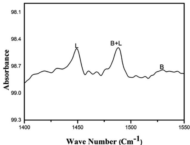
Fig. 5 Pyridine IR spectrum of 2.5% Bi<sub>2</sub>O<sub>3</sub>/ZrO<sub>2</sub> catalyst.
