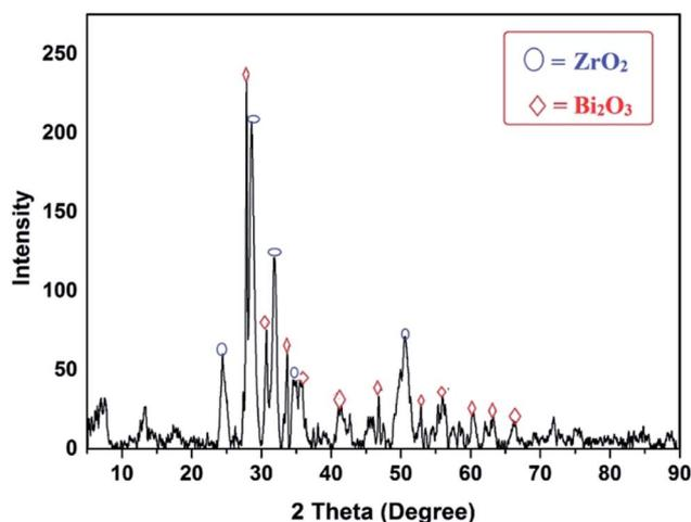
Fig. 1 Powder X-ray diffractogram of 2.5%  $\text{Bi}_2\text{O}_3-\text{ZrO}_2$  catalyst.
