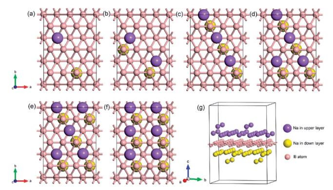
Fig. 6 The most stable structures at different x values of  $Na_xB_{24}$ ; the x value is an even number ranging from 2 to 14 for (a)–(g), respectively.
