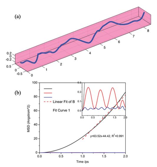
Fig. 10 Calculated trajectories (a) and MSD in three directions (b) of a sodium ion during the last 2 ps by AIMD simulation.
