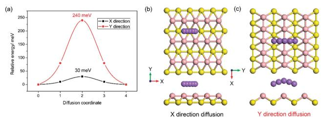
Fig. 9 Energy profile of sodium diffusion in the *X* direction in the furrows and the *Y* direction crossing ridges (a); top and side views of sodium diffusion in the furrows (b) and crossing the ridges (c).
