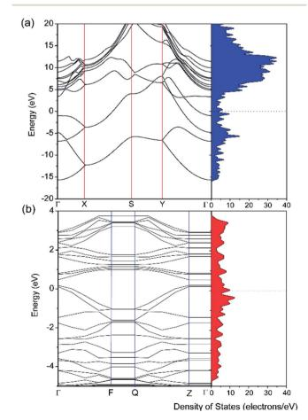
Fig. 3 Calculated band structure and density of states (DOS) of (a) pristine borophene and (b) borophene with a single vacancy defect. The Fermi level is set at 0 eV
