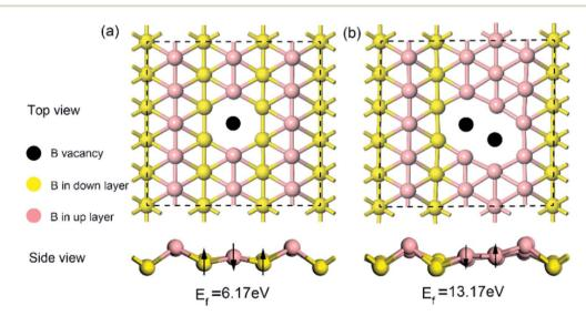
Fig. 2 Top and side views of the optimized structures for (a) borophene with a single vacancy defect and (b) borophene with a double vacancy defect.
