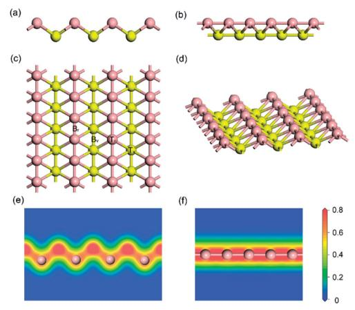
Fig. 1 Side views (a) and (b); top view (c) and 3D view (d) of the optimized structure for  $(5 \times 3)$  monolayer borophene; electron densities (unit: electrons per  $\mathring{A}^3$ ) in (e) the [100] and (f) the [010] direction. For ease of visualization, the boron atoms in different atomic layers are marked in either pink or yellow.
