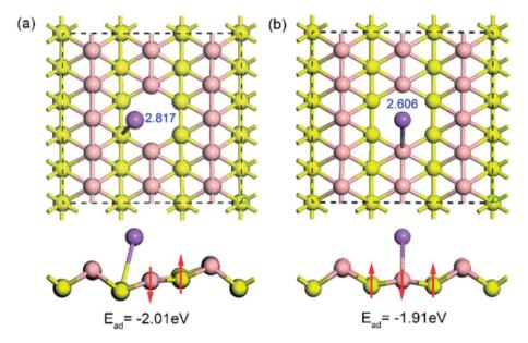
Fig. 5 Top and side views of the optimized structures for a sodium atom adsorption on a 5 × 3 borophene supercell with a single vacancy defect.
