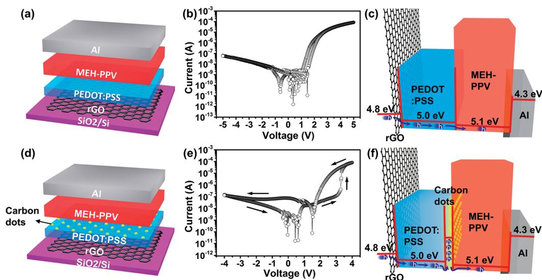
Fig. 2 (a) Schematic structure, (b) typical *I*–*V* characteristics and (c) energy band diagram of the rectifying device. (d) Schematic structure, (e) typical *I*–*V* characteristics (the arrows represent the sweep directions) and (f) energy band diagram of the rectifying memory device.
