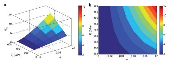
The relative modulus as a function of the " $\phi_i$ " and " $E_i$ " parameters at  $E_m = 2$  GPa,  $\phi_f = 0.01$  and  $E_f = 1000$  GPa: (a) 3D and (b) contour plots.
