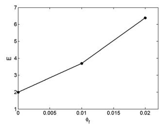
Fig. 2 Moduli predicted by the simplified Kolarik model at  $E_{\rm m}=2$  GPa,  $E_{\rm f}=1000$  GPa, R=10 nm, l=10  $\mu{\rm m}$  and t=5 nm.
