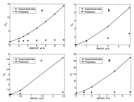
Fig. 5 Overprediction of the developed model for (a) PA6/MWCNT,<sup>40</sup> (b) PVA/MWCNT,<sup>41</sup> (c) polypropylene/MWCNT<sup>42</sup> and (d) PA6/MWCNT<sup>43</sup> samples.
