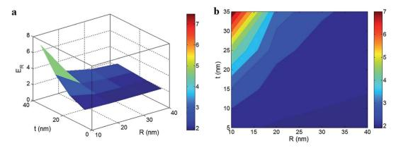
Fig. 7 (a) 3D and (b) contour plots to describe the influence of the "R" and "t" parameters on the calculated relative modulus at average values of  $E_{\rm m} = 2$  GPa,  $\phi_{\rm f} = 0.01$ ,  $E_{\rm f} = 1000$  GPa and  $E_{\rm i} = 100$  GPa.
