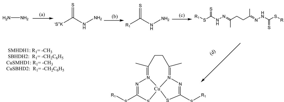
Scheme 7 Synthesis of the copper complexes from bis(dithiocarbamate) ligands. Reagents and conditions: (a) CS<sub>2</sub>, KOH, EtOH, 0 °C, 1 h; (b) CH<sub>3</sub>I or PhCH<sub>2</sub>Cl, EtOH, 0 °C, 5 h; (c) for SMHDH<sub>2</sub> (2,5-hexanedione, EtOH, 79 °C, 1 h), for SBHDH<sub>2</sub> (2,5-hexanedione, EtOH, 79 °C, 5 min) and (d) for CuSMHD [Cu(OAc)<sub>2</sub>·H<sub>2</sub>O, MeOH, 65 °C, 1 h], for CuSBHD [Cu(OAc)<sub>2</sub>, acetonitrile, r.t, 1 h].
