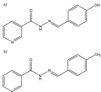
Fig. 11 Chemical structure of the synthesized corrosion inhibitors: (a) *N'*-(4-hydroxybenzylidene)nicotinic hydrazone (HBNH), and (b) *N'*-(4-methylbenzylidene)nicotinic hydrazone (MBNH).
