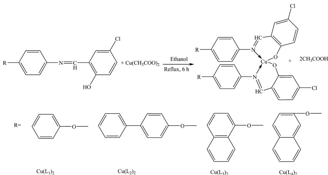
Scheme 1 Synthesis of Cu(II) complexes [ $Cu(L_1)_2$ – $Cu(L_4)_2$ ].
