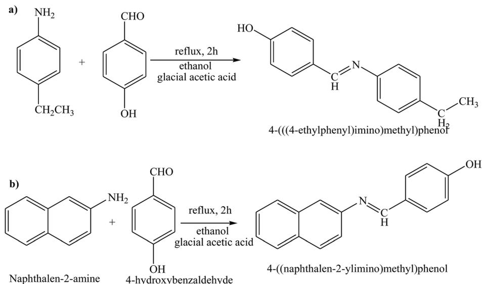
Scheme 25 Reaction pathway showing the formation (*E*)-4-(((naphthalen-2-ylimino)methyl)phenol Schiff base.
