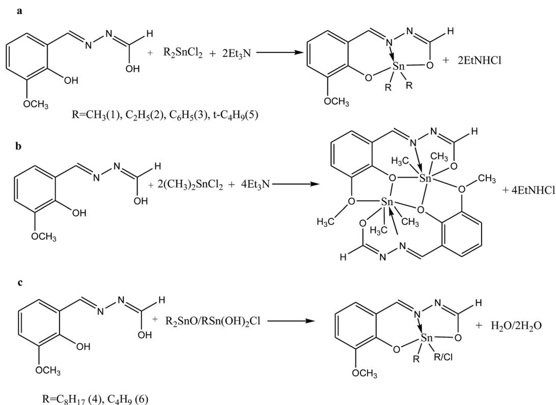
Scheme 3 Synthesis of Schiff base complexes (a–c).
