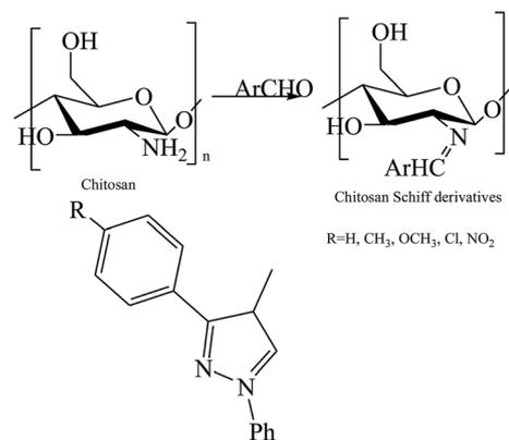
Scheme 17 Synthesis of chitosan Schiff bases (ChBs).
