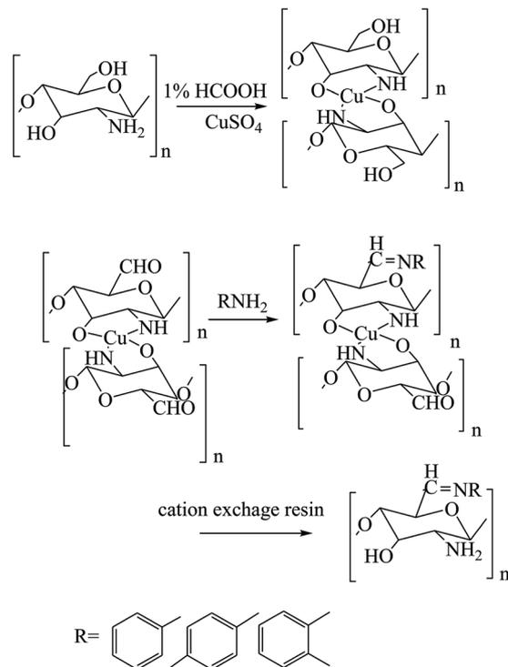
Scheme 16 Synthesis of C6-Schiff bases of chitosan derivatives.
