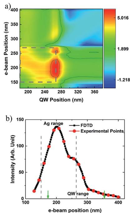
Fig. 7 (a) Calculated power distribution ( $P_{inj}$ ) on log scale in the QW region injected by z-dipole induced LSP, and (b) calculated CL intensity for each e-beam position with a step of 2 nm (black) and corresponding experimental points (red). The color bar shows the log scale of the normalized electric field.
