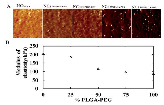
Fig. 2 Elastic modulus of NCs<sub>PLGA</sub>, NCs<sub>25% PLGA-PEG</sub>, NCs<sub>50% PLGA-PEG</sub>, NCs<sub>75% PLGA-PEG</sub> and NCs<sub>100% PLGA-PEG</sub> in suspension. (A) Images of the elastic modulus of NCs, with the weight percentage of PLGA-PEG gradually increasing (0, 25, 50, 75, 100%) in the formulation. (B) Plot of the corresponding nanocapsules' bulk modulus as a function of PLGA-PEG percentage.
