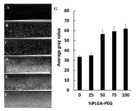
Fig. 5 In vitro ultrasound images of different nanocapsule suspensions. (A) Degassed deionized water (control), (B) NCs<sub>PLGA</sub>, (C) NCs<sub>25% PLGA-PEG</sub>, (D) NCs<sub>50% PLGA-PEG</sub>, (E) NCs<sub>75% PLGA-PEG</sub>, (F) NCs<sub>100% PLGA-PEG</sub>, (G) Quantitative analysis of echo-signal intensity with different NCs.
