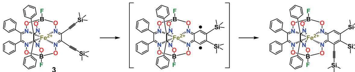
Scheme 5 Plausible pathway of chemical transformations of the *vic*-diethynyl-substituted iron(II) clathrochelate  $\text{FeBd}_2(((\text{Me}_3\text{Si})\text{C}\equiv\text{C})_2\text{Gm})(\text{BF}_2)$  (3) as a reactive intermediate.
