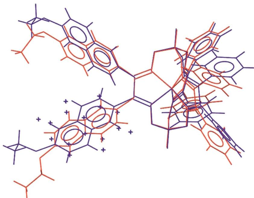
Fig. 4 Overlaid clathrochelate molecules in the solvent-containing and solvent-free solvatomorphs FeBd<sub>2</sub>((EtONaphth)<sub>2</sub>Gm)(BF)<sub>2</sub>·3CH<sub>2</sub>Cl<sub>2</sub> (1·3CH<sub>2</sub>Cl<sub>2</sub>, in red) and FeBd<sub>2</sub>((EtONaphth)<sub>2</sub>Gm)(BF)<sub>2</sub> (1, in blue).
