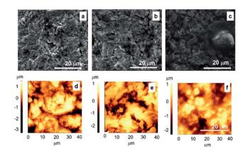
Fig. 5 SEM (a–c) and AFM (d–f) micrographs of the Gum alloy (a and d) functionalized with GNP (b and e), and GNP–SS (c and f) by MAPLE (266 nm, 600 mJ cm $^{-2}$ ). The scanned area by AFM was 40  $\times$  40  $\mu m^2$ . Scale bar: 20  $\mu m$ .
