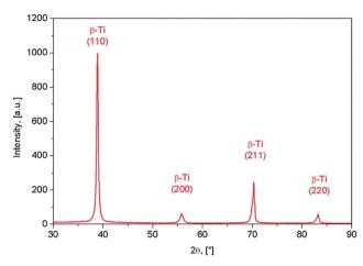
Fig. 2 XRD spectra of Ti-31.7Nb-6.21Zr-1.4Fe-0.16O (% wt) Gumtupe alloy.
