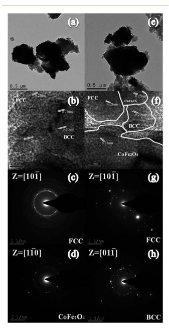
Fig. 3 (a and e) TEM and (b and f) HRTEM images of (a-c) as-milled and (d-h) as-annealed FeCoNiSi<sub>0.3</sub>Al<sub>0.4</sub> HEA powders. The SAED patterns (c) and (d, g and h) for the samples.
