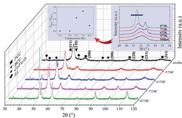
Fig. 8 XRD patterns of the as-milled and as-annealed (573–873 K) FeCoNiSi<sub>0.3</sub>Al<sub>0.4</sub> alloy powders, and the inset present the detailed scans in the range of  $2\theta = 49$ – $56^\circ$ . The relative content of BCC to FCC ( $A_{BCC}/A_{FCC}$ ) for different anneal temperature are also presented in the illustration.
