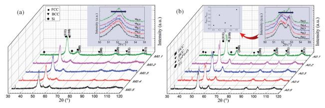
Fig. 1 XRD patterns of (a) as-milled and (b) as-annealed FeCoNiSi<sub>x</sub>Al<sub>0.4</sub> HEA powders, and the detailed scans in the range of  $2\theta = 50-55^{\circ}$  are presented in the illustration. The change in area ratio ( $A_{BCC}/A_{FCC}$ ) for the as-annealed HEA powders is also presented in the illustration. All alloys are composed of BCC and FCC phase except a small amount of Si remained indicating the formation of high entropy alloy.
