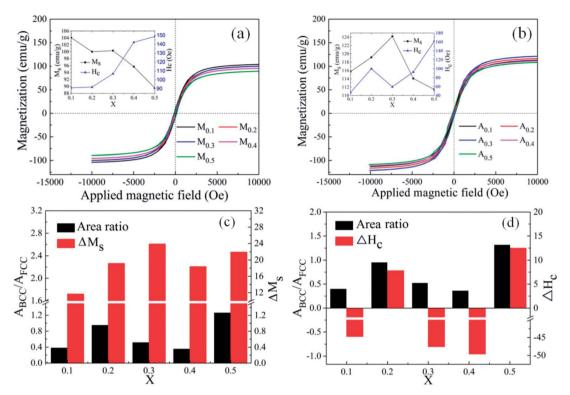
Fig. 4 Hysteresis loops of (a)  $M_{0.1-0.5}$  and (b)  $A_{0.1-0.5}$ , and the illustrations present the change in magnetic parameters ( $H_c$  and  $M_s$ ) of both kinds of alloy powders. (c-d) is the area ratio ( $A_{BCC}/A_{FCC}$ ),  $\Delta M_s$  ( $M_s$  ( $A_x$ ) -  $M_s$  ( $M_x$ )), and  $\Delta H_c$  ( $H_c$  ( $H_c$  ( $H_x$ )) for different alloy powders. Wherein Xrepresents the molar amount of Si in FeCoNiSixAl<sub>0.4</sub> alloy powders.
