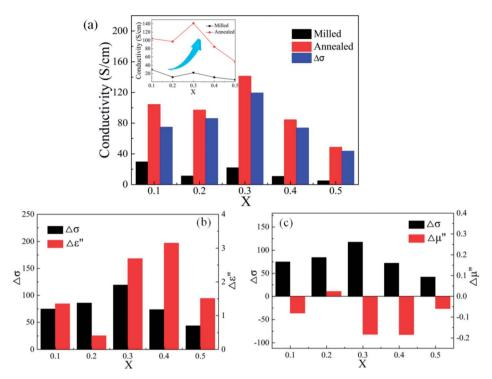
Fig. 6 (a) The change in the conductivity of as-milled, as-annealed alloy powders and the increment ( $\Delta\sigma$ ) are presented. (b andc) is the  $\Delta\sigma$ ,  $\Delta\varepsilon''$  (at 18 GHz), and  $\Delta\mu''$  (at 10 GHz) for different alloy powders. Wherein X represents the molar amount of Si in FeCoNiSi<sub>x</sub>Al<sub>0.4</sub> alloy powders.
