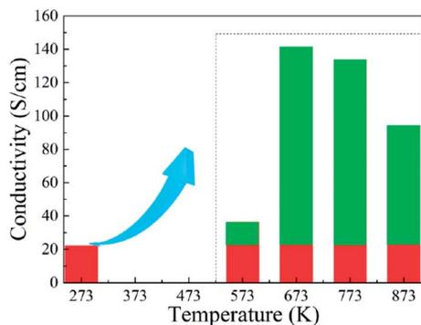
Fig. 10 Effect of annealing temperature on the conductivity of FeCoNiSi<sub>0.3</sub>Al<sub>0.4</sub> alloy powders.
