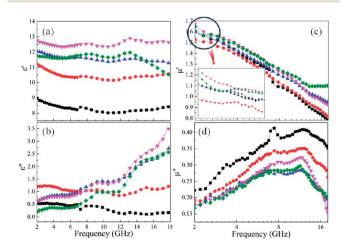
Fig. 9 Frequency dependence of (a)  $\epsilon'$ , (b)  $\epsilon''$ , (c)  $\mu'$ , and (d)  $\mu''$  for the as-annealed (573–873 K) FeCoNiSi<sub>0.3</sub>Al<sub>0.4</sub>–paraffin composites. The symbols of  $\blacksquare$ ,  $\bullet$ ,  $\blacktriangle$ ,  $\blacktriangledown$  and  $\bullet$  denote the milled, 573 K, 673 K, 773 K and 873 K composites, respectively.
