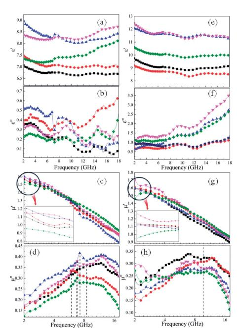
Fig. 5 Frequency dependence of (a and e)  $\varepsilon'$ , (b and f)  $\varepsilon''$ , (c and g)  $\mu'$ , and (d and h)  $\mu''$  for the (a–d) as-milled and (e–h) as-annealed FeCoNiSi<sub>x</sub>Al<sub>0.4</sub>—paraffin composites. The symbols of  $\blacksquare$ ,  $\bigcirc$ , and  $\blacklozenge$  denote the x = 0.1, 0.2, 0.3, 0.4, and 0.5 composites, respectively.
