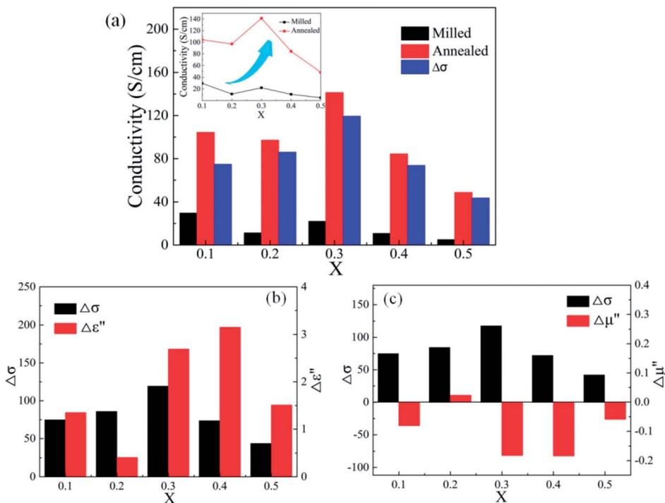
Fig. 6 (a) The change in the conductivity of as-milled, as-annealed alloy powders and the increment ( $\Delta\sigma$ ) are presented. (b and c) is the  $\Delta\sigma$ ,  $\Delta\epsilon''$  (at 18 GHz), and  $\Delta\mu''$  (at 10 GHz) for different alloy powders. Wherein X represents the molar amount of Si in FeCoNiSi<sub>x</sub>Al<sub>0.4</sub> alloy powders.
