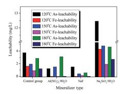
Fig. 8 The As-leachability with various mineralizers (Na<sub>2</sub>SiO<sub>3</sub>·9H<sub>2</sub>O, Al(NO<sub>3</sub>)<sub>3</sub>·9H<sub>2</sub>O, and NaF) and at various temperatures (120 °C, 150 °C, and 180 °C) for 25 h.
