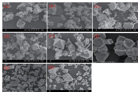
Fig. 11 SEM images for solid precipitates with various temperatures and mineralizers: (a) 120 °C-H<sub>2</sub>O control group, (b) 150 °C-H<sub>2</sub>O control group, (c) 180 °C-H<sub>2</sub>O control group, (d) 120 °C-NaF modified, (e) 150 °C-NaF modified, (f) 180 °C-NaF modified, (g) 180 °C-Na<sub>2</sub>SiO<sub>3</sub>·9H<sub>2</sub>O modified, and (h) 180 °C-Al (NO<sub>3</sub>)<sub>3</sub>·9H<sub>2</sub>O modified for 25 h.
