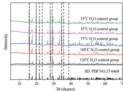
Fig. 5 XRD patterns of samples at various temperatures ( $35^\circ\text{C}$ ,  $55^\circ\text{C}$ ,  $75^\circ\text{C}$ ,  $100^\circ\text{C}$ , and  $120^\circ\text{C}$ ) with an Fe/As molar ratio of 2, and pH 2.5 for 25 h.
