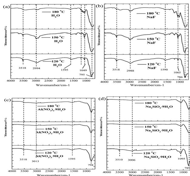
**Fig. 10** FT-IR spectra of an arsenate-containing solid after hydrothermal mineralization with the various mineralizers (a)  $\text{H}_2\text{O}$ -control group, (b) NaF-modified, (c)  $\text{Al}(\text{NO}_3)_3 \cdot 9\text{H}_2\text{O}$ -modified, (d) and  $\text{Na}_2\text{SiO}_3 \cdot 9\text{H}_2\text{O}$ -modified, and at various hydrothermal mineralization temperatures (120 °C, 150 °C, and 180 °C) for 25 h.
