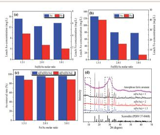
Fig. 1 Effect of the Fe/As molar ratio and the iron sources (a) Fe(II)/As and (b) Fe(III)/As on leaching As-concentration and Fe-concentration, (c) the As-removal rate for solid samples obtained at pH 2.5 at 95 °C for 5 h, and (d) XRD spectra of scorodite samples obtained at various Fe/As molar ratios, pH 2.5, and 95 °C for 5 h.
