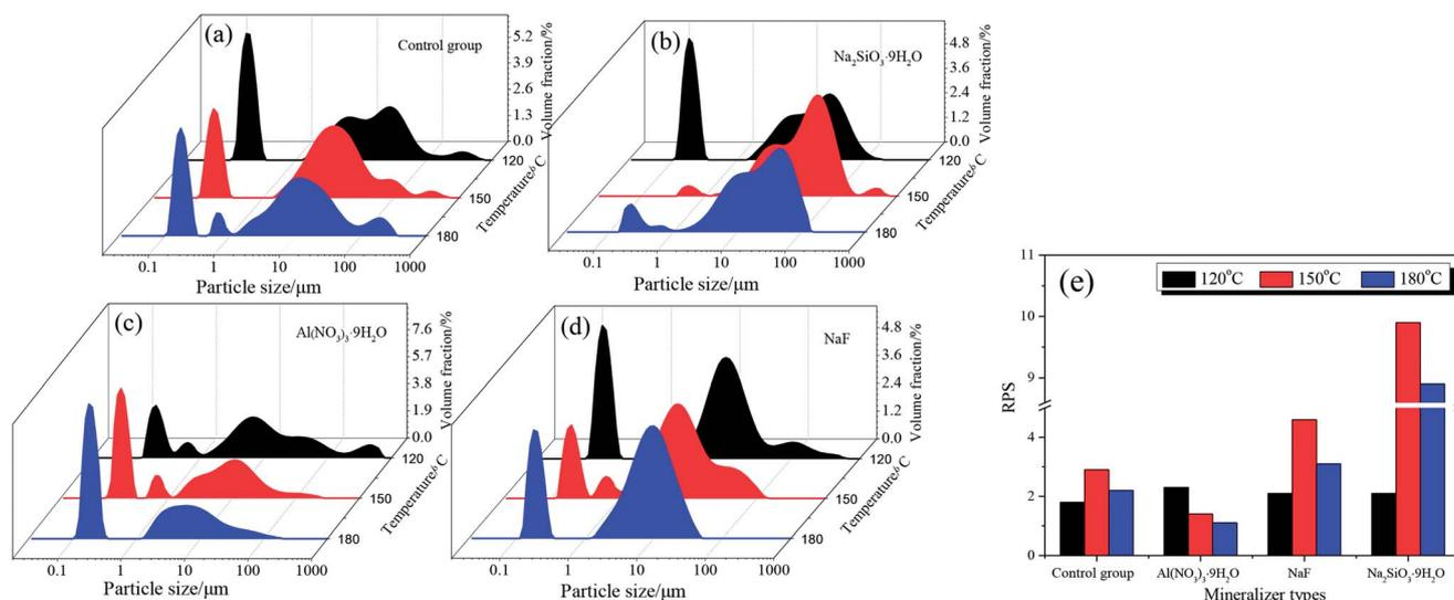
Fig. 12 The particle size distribution for solid precipitates under various temperature and mineralizers (a) H<sub>2</sub>O control group, (b) Na<sub>2</sub>SiO<sub>3</sub>·9H<sub>2</sub>O modified, (c) Al (NO<sub>3</sub>)<sub>3</sub>·9H<sub>2</sub>O modified, (d) NaF modified, and (e) RPS.
