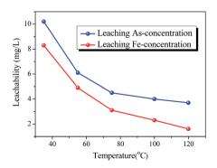
Fig. 4 The effect of aging temperature on leaching As-concentration (EPA-TCLP methods) for solid samples. The samples were obtained at 95 °C with an Fe/As molar ratio of 2, and pH 2.5.
