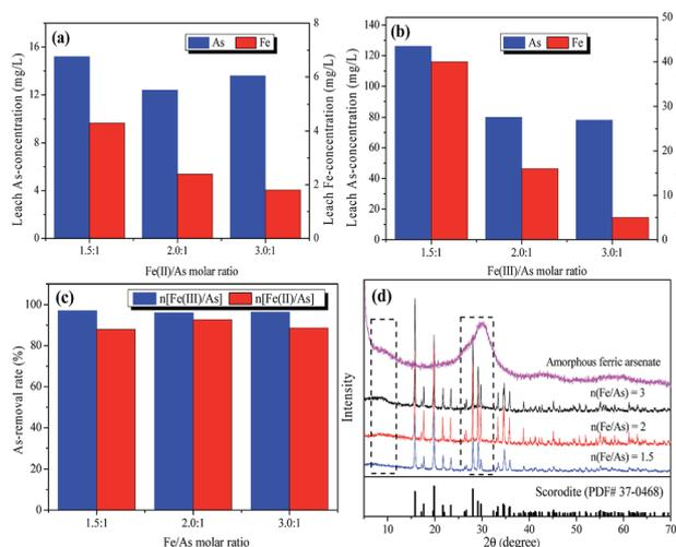
**Fig. 1** Effect of the Fe/As molar ratio and the iron sources (a) Fe(II)/As and (b) Fe(III)/As on leaching As-concentration and Fe-concentration, (c) the As-removal rate for solid samples obtained at pH 2.5 at  $95^\circ\text{C}$  for 5 h, and (d) XRD spectra of scorodite samples obtained at various Fe/As molar ratios, pH 2.5, and  $95^\circ\text{C}$  for 5 h.
