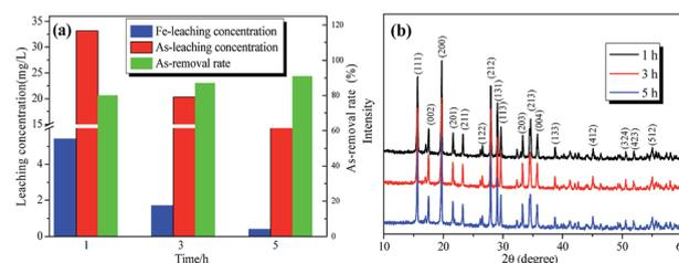
**Fig. 2** Effect of the reaction time on (a) As or Fe-leachability and As-removal rate, (b) the XRD pattern of the scorodite samples, which was obtained at an Fe/As molar ratio of 2, a pH of 2.5, and  $95^\circ\text{C}$ .
