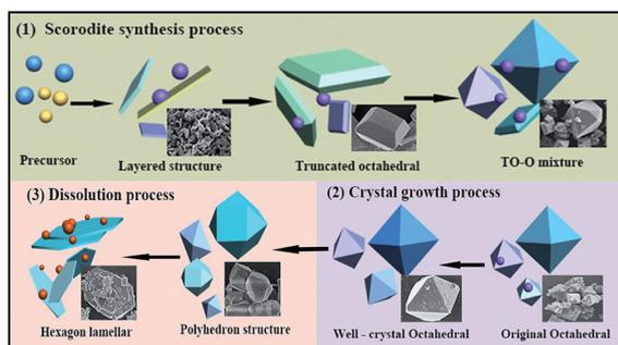
Fig. 13 Diagram of scorodite crystal behavior process.
