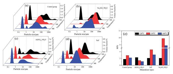
Fig. 12 The particle size distribution for solid precipitates under various temperature and mineralizers (a) H<sub>2</sub>O control group, (b) Na<sub>2</sub>SiO<sub>3</sub>·9H<sub>2</sub>O modified, (c) Al (NO<sub>3</sub>)<sub>3</sub>·9H<sub>2</sub>O modified, (d) NaF modified, and (e) RPS.
