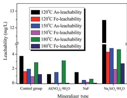
Fig. 8 The As-leachability with various mineralizers ( $\text{Na}_2\text{SiO}_3 \cdot 9\text{H}_2\text{O}$ ,  $\text{Al}(\text{NO}_3)_3 \cdot 9\text{H}_2\text{O}$ , and NaF) and at various temperatures (120 °C, 150 °C, and 180 °C) for 25 h.
