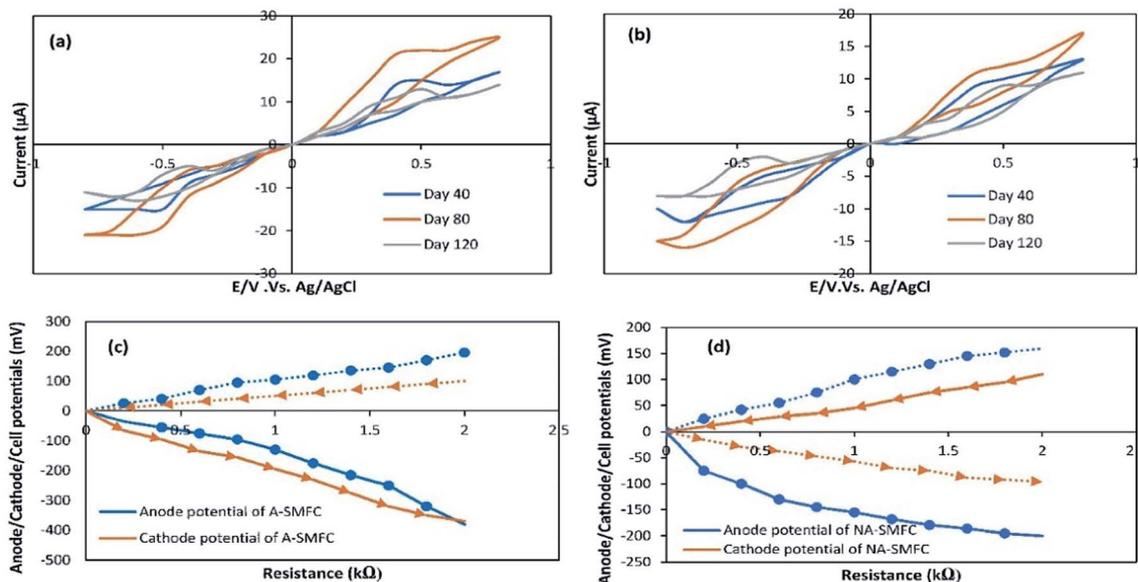
Fig. 4 Cyclic voltammograms for (a) A-SMFCs and (b) NA-SMFCs operating over the range of -0.8 to +0.8  $\mu$ A. Cell potentials (solid lines show cell potentials, dashed dots show anode potentials, and dashed arrows show cathode potentials) for A-SMFCs (c) and NA-SMFCs (d).
