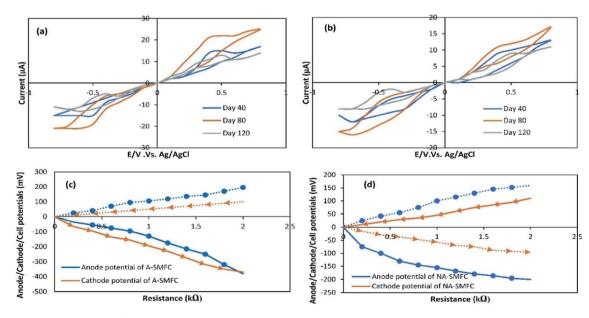
Fig. 4 Cyclic voltammograms for (a) A-SMFCs and (b) NA-SMFCs operating over the range of -0.8 to +0.8  $\mu$ A. Cell potentials (solid lines show cell potentials, dashed dots show anode potentials, and dashed arrows show cathode potentials) for A-SMFCs (c) and NA-SMFCs (d).
