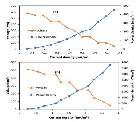
Fig. 3 Polarization plots for (a) A-SMFCs and (b) NA-SMFCs operated over the external resistance range of 60  $\Omega$  to 2 k $\Omega$ .
