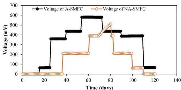
Fig. 2 Voltage generation trends for A-SMFCs and NA-SMFCs.
