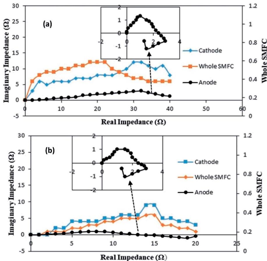
Fig. 5 Nyquist curves for the cathode, anode and whole SMFC: (a) A-SMFC; and (b) NA-SMFC. The insets represent the anode response.
