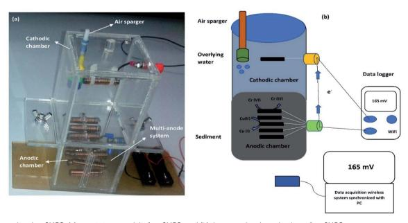
Fig. 1 A two chamber SMFC: (a) a prototype model of an SMFC: and (b) the operational mechanism of an SMFC.
