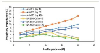
Fig. 6 Nyquist plots indicating EIS data fitted to the ECM model on days 40, 80 and 120 for the A-SMFC and NA-SMFC.
