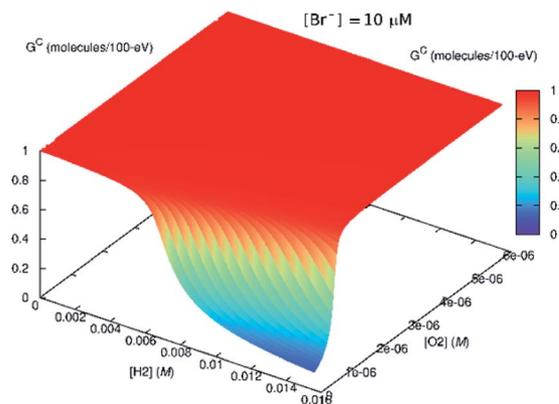
Fig. 8 Effect of bromide ( $[\text{Br}^-] = 10 \mu\text{M}$ ) on the steady-state  $G^C$  value. If  $\text{H}_2$  is present in the system initially, the scavenging effect of  $\text{Br}^-$  diminishes.
