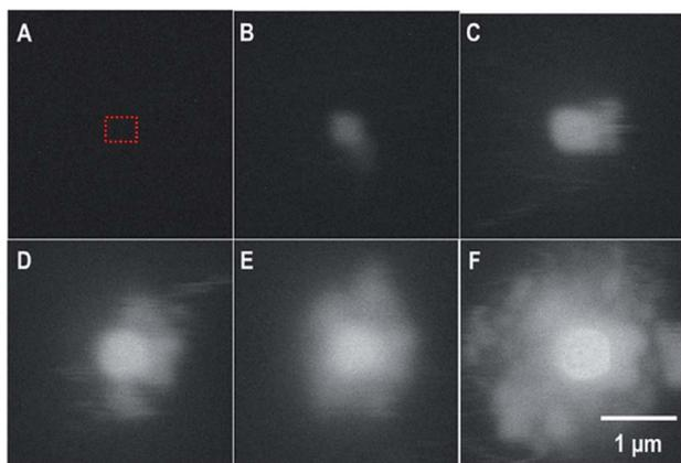
Fig. 5 SEM-BSE images from the *in situ* LC showing the formation of a uranyl peroxide over time: (A) 0 s; (B) 78 s; (C) 194 s; (D) 314 s; (E) 479 s; and (F) 640 s. The irradiation occurred over a  $< 1 \mu\text{m}^2$  region in the center. The blurring is the result of the fast scan to capture the image without inducing excess irradiation to the area. The dotted red box represents the region that was irradiated.
