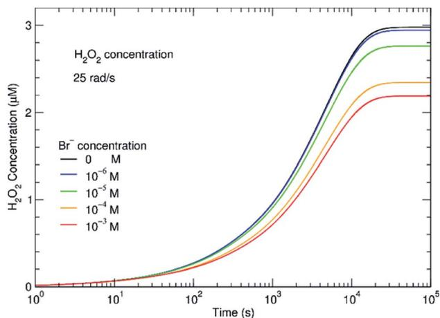
Fig. 4 Effect of bromide on the steady-state concentration of  $\text{H}_2\text{O}_2$  at a dose rate of  $0.25 \text{ Gy s}^{-1}$ . Within minutes, the  $\text{H}_2\text{O}_2$  concentration reaches a steady state concentration that depends on the initial  $\text{Br}^-$  added.
