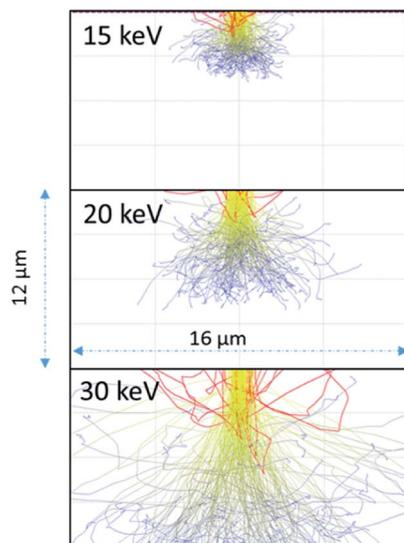
Fig. 3 Anticipated electron scattering through water for a 1  $\mu\text{m}$  wide beam at 15, 20, and 30 keV using the CASINO program.<sup>10</sup> The red lines are backscattered electrons; the yellow are higher energy electrons leading to radiolytic events. The blue lines are scattered lower energy electrons although these electrons would still induce radiolytic events.
