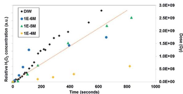
Fig. 6 *In situ* microscopy measurement of uranyl peroxide formation with time and  $\text{Br}^-$  concentration (measurement method described in the ESI† section). The dotted line shows the dose (measured in Greys) estimated in the irradiated region with time.
