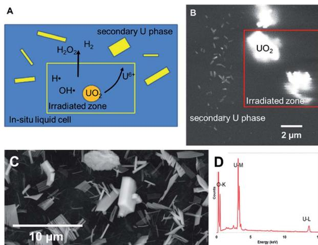
Fig. 9 (A) Schematic showing the effect of localised electron irradiation on a solution containing  $\text{UO}_2$  particles. (B) SEM-BSE image showing the formation of studtite during irradiation of  $\text{UO}_2$  particles in solution. The irradiated zone is marked within the red outlined box. (C) SEM image of studtite formed from the alteration of irradiated U fuel in the K-Basins at the Hanford site, Washington, USA. (D) X-Ray energy dispersive analysis of the phase.
