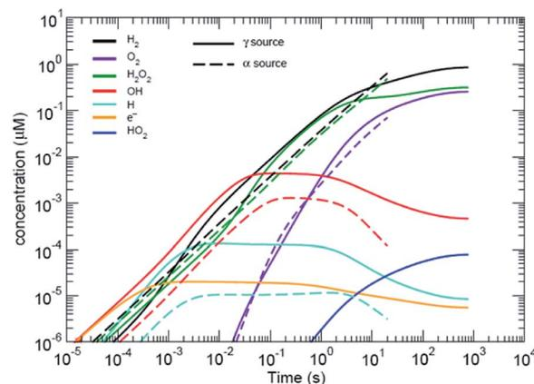
Fig. 2 Predicted radiolytic species production rates for both  $\alpha$  and  $\beta/\gamma$  radiation. The black lines corresponds to using the rate constants from ref. 15.  $\alpha$ -Radiation results in a continuous production rate of  $\text{H}_2$  and  $\text{H}_2\text{O}_2$ ; whereas, production under  $\beta,\gamma$ -radiation reaches a steady-state condition.
