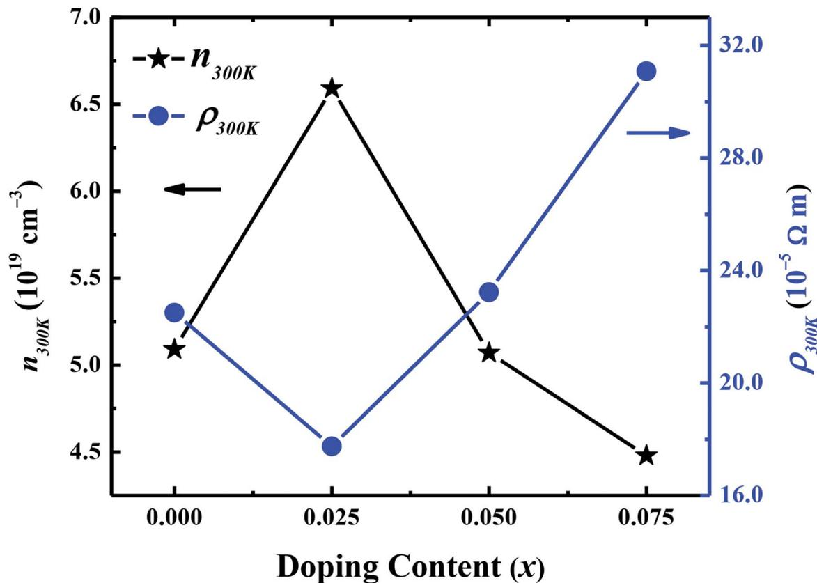
Fig. 6 Room temperature carrier concentration ( $n_{300 \text{ K}}$ ) and electrical resistivity ( $\rho_{300 \text{ K}}$ ) as a function of doping ( $x$ ) for  $\text{Ca}_{3-2x}\text{Na}_{2x}\text{Co}_{4-x}\text{W}_x\text{O}_9$  ( $0 \leq x \leq 0.075$ ) samples.
