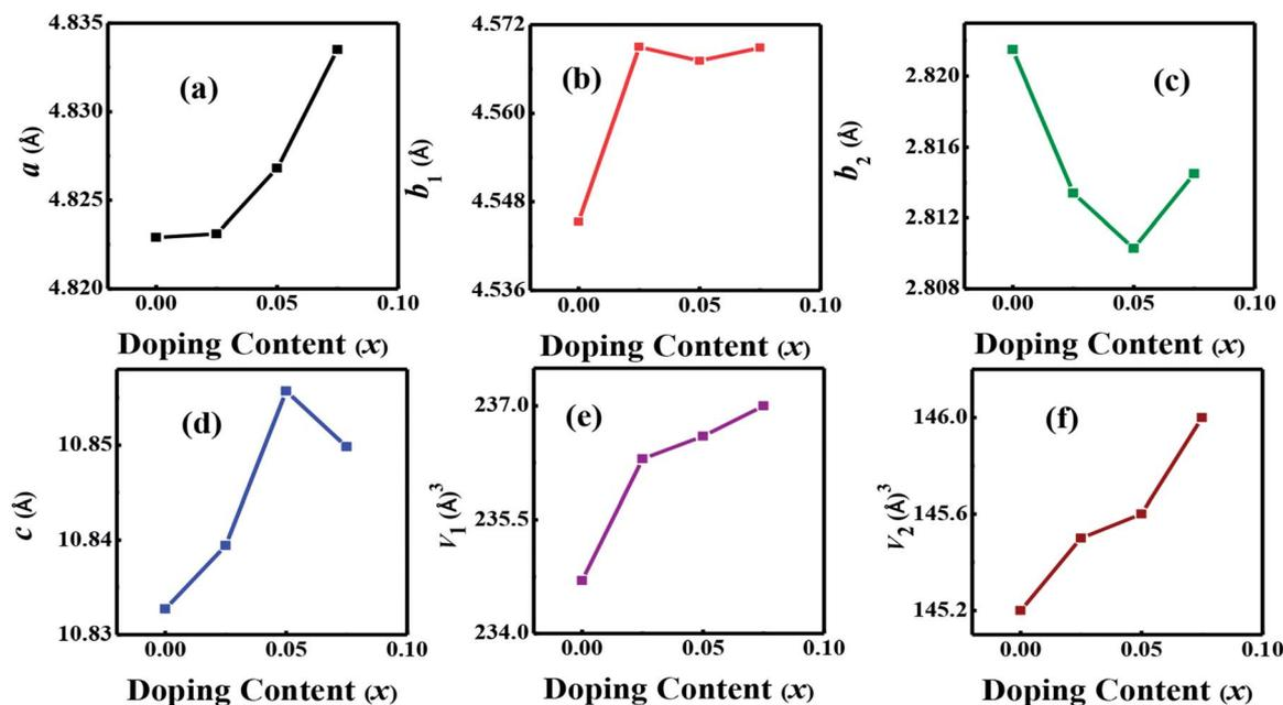
**Fig. 2** Structural parameters  $a$ ,  $b_1$ ,  $b_2$ ,  $c$ ,  $V_1$  and  $V_2$  as a function of doping content ( $x$ ) for  $\text{Ca}_{3-2x}\text{Na}_{2x}\text{Co}_{4-x}\text{W}_x\text{O}_9$  ( $0 \leq x \leq 0.075$ ) series.
