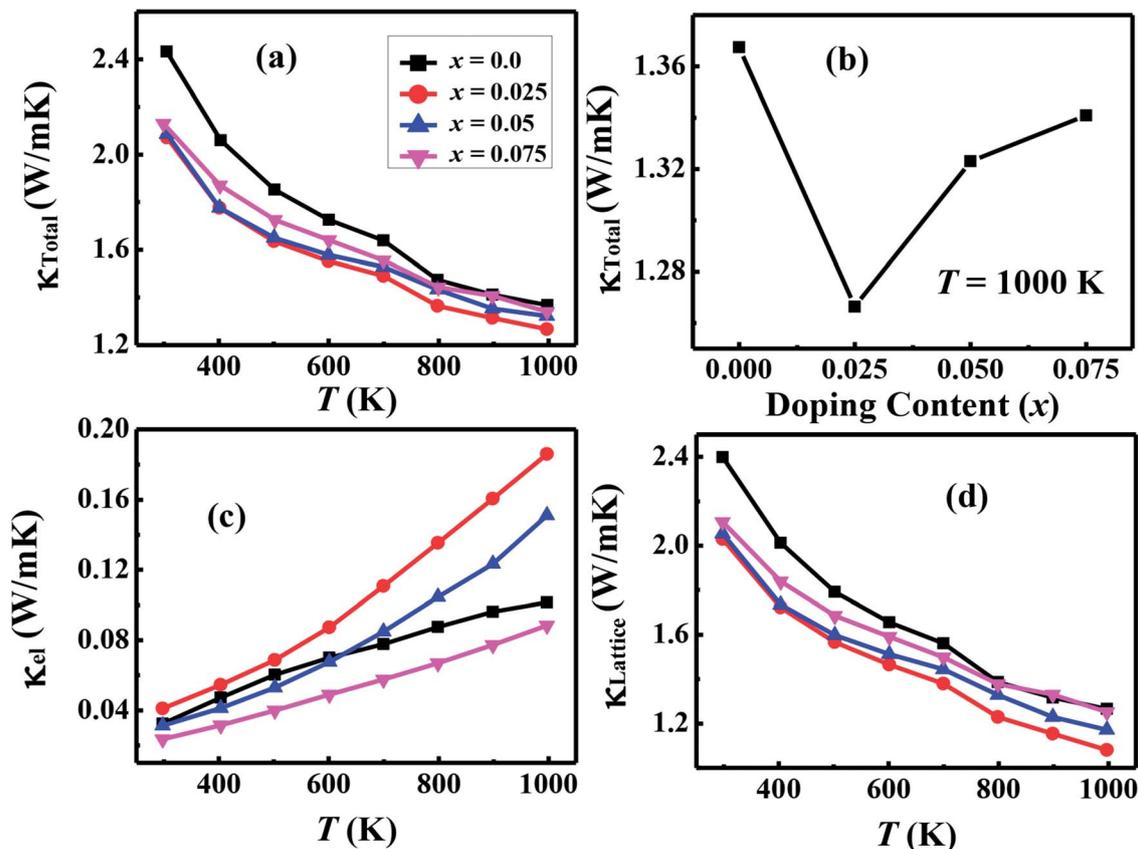
Fig. 9 (a) Total thermal conductivity ( $\kappa_{\text{Total}} = \kappa_{\text{el}} + \kappa_{\text{Lattice}}$ ); (b) doping content ( $x$ ) dependence of  $\kappa_{\text{Total}}$  at 1000 K; (c) electronic part of thermal conductivity ( $\kappa_{\text{el}}$ ) and (d) lattice part of thermal conductivity ( $\kappa_{\text{Lattice}}$ ) for  $\text{Ca}_{3-2x}\text{Na}_{2x}\text{Co}_{4-x}\text{W}_x\text{O}_9$  ( $0 \leq x \leq 0.075$ ) samples as a function of temperature.
