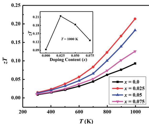
Fig. 10 Thermoelectric figure of merit ( $zT$ ) for  $\text{Ca}_{3-2x}\text{Na}_{2x}\text{Co}_{4-x}\text{W}_x\text{O}_9$  ( $0 \leq x \leq 0.075$ ) samples as a function of temperature; inset shows doping content ( $x$ ) dependence of  $zT$  at 1000 K.
