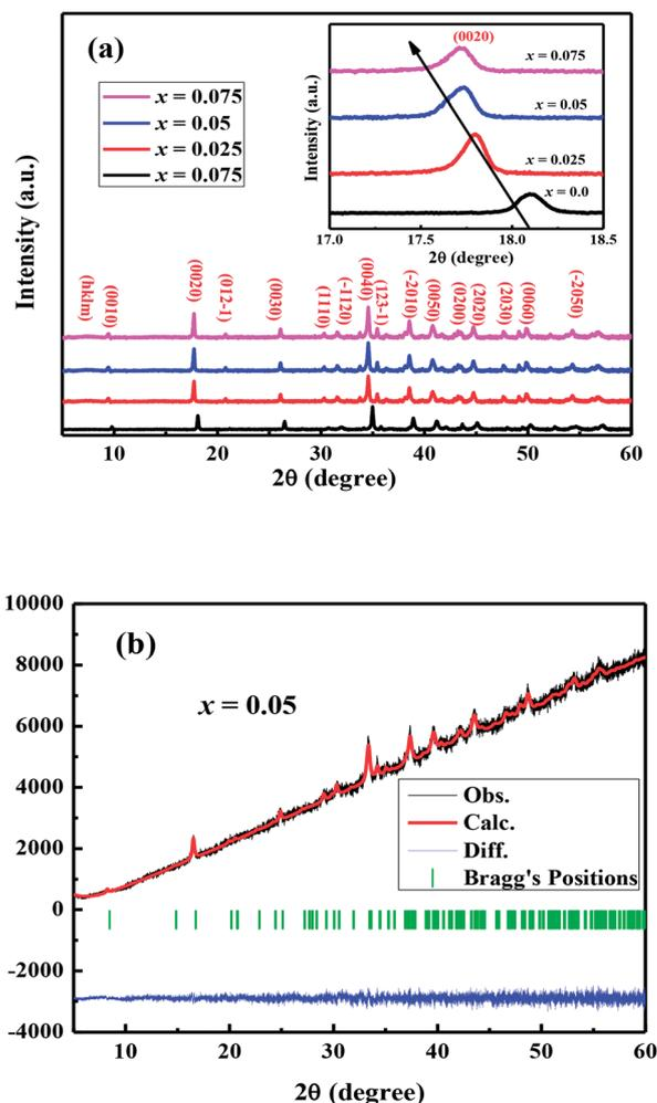
Fig. 1 (a) XRD patterns of  $\text{Ca}_{3-2x}\text{Na}_{2x}\text{Co}_{4-x}\text{W}_x\text{O}_9$  ( $0 \leq x \leq 0.075$ ) samples; inset: the shift of (0020) peaks with change of doping content ( $x$ ). (b) Rietveld refined XRD pattern of  $\text{Ca}_{2.9}\text{Na}_{0.1}\text{Co}_{3.95}\text{W}_{0.05}\text{O}_9$  sample.
