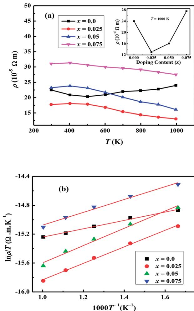
Fig. 5 (a) Electrical resistivity ( $\rho$ ) for  $\text{Ca}_{3-2x}\text{Na}_{2x}\text{Co}_{4-x}\text{W}_x\text{O}_9$  ( $0 \leq x \leq 0.075$ ) samples as a function of temperature; inset shows doping content ( $x$ ) dependence of  $\rho$  at 1000 K. (b) Linear fits of  $\ln(\rho/T)$  vs.  $1000/T$  for  $\text{Ca}_{3-2x}\text{Na}_{2x}\text{Co}_{4-x}\text{W}_x\text{O}_9$  ( $0 \leq x \leq 0.075$ ) samples.
