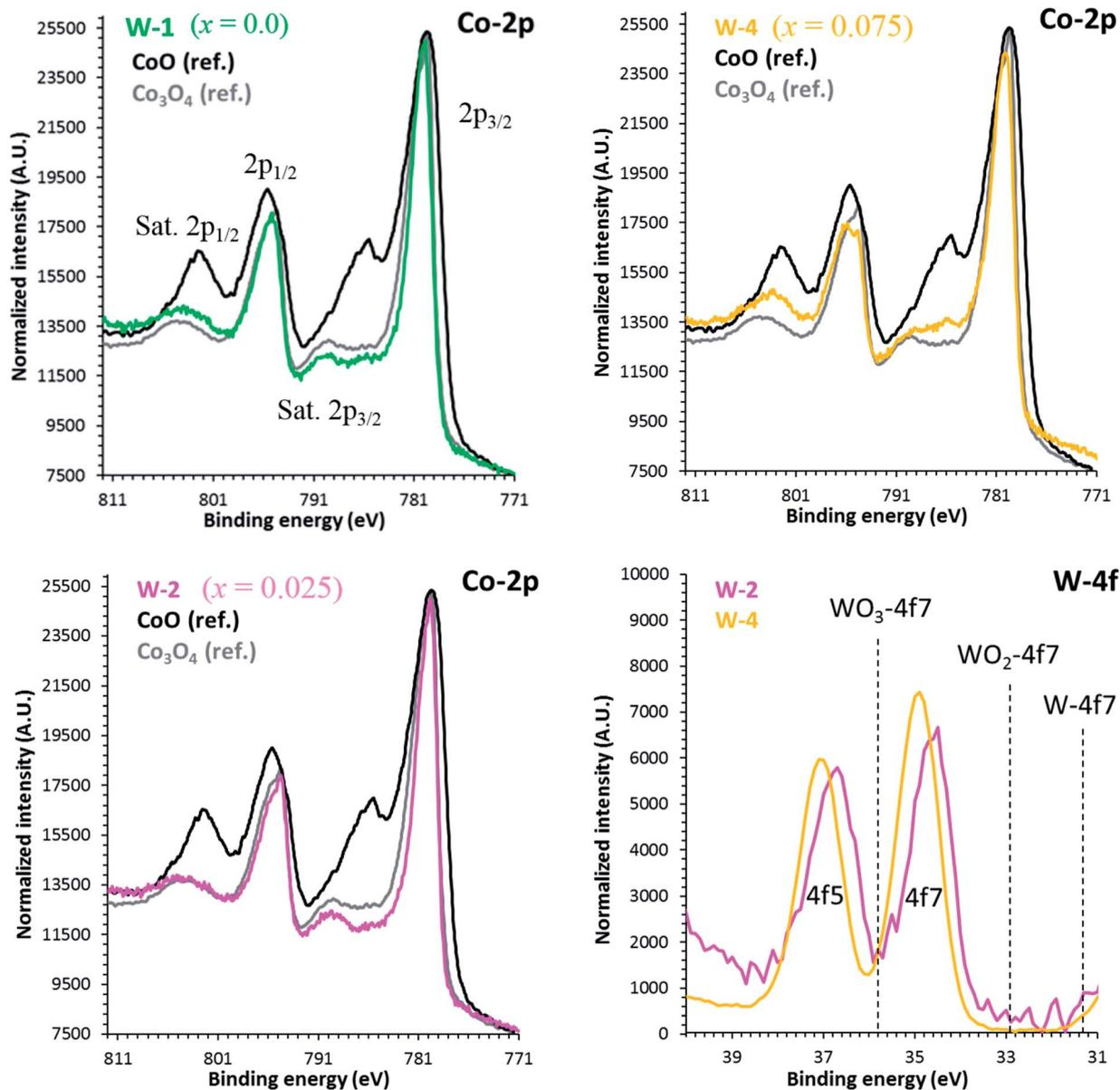
Fig. 4 High resolution XPS spectra of Co 2p and W 4f for C-349 doped samples. Reference positions are taken from the NIST database.
