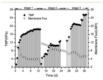
Fig. 3 Transmembrane pressure and membrane flux profile.
