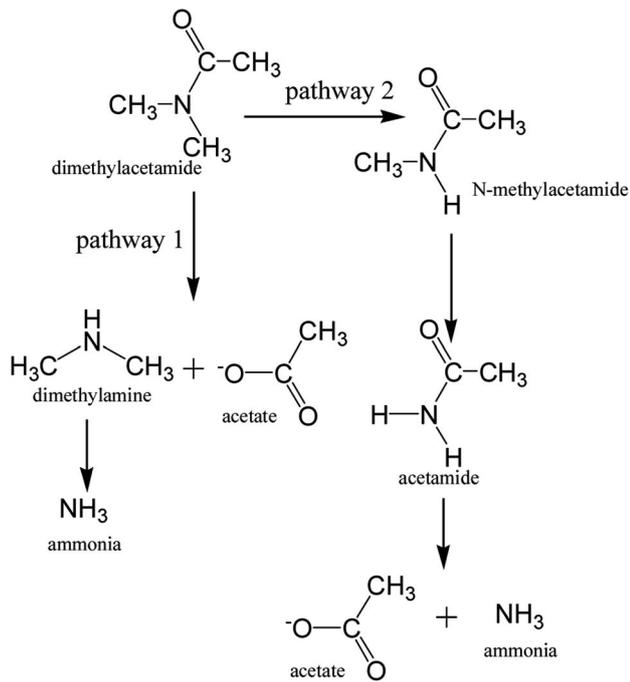
Fig. 7 Two proposed pathways for DMAC biodegradation.
