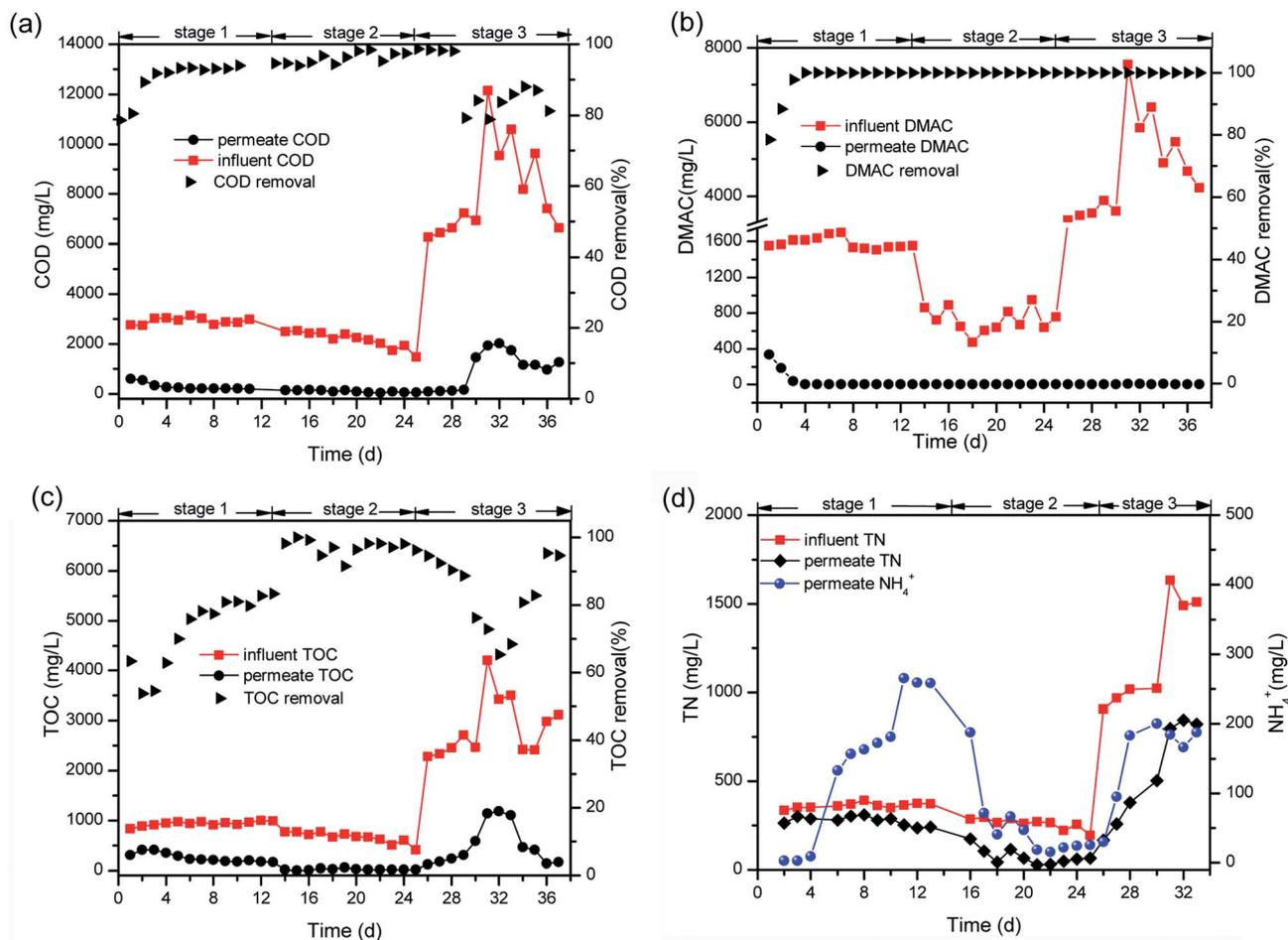
Fig. 2 Variation of treatment indicators in the MBR effluent including (a) COD, (b) DMAC, (c) TOC, and (d) NH<sub>4</sub><sup>+</sup>, and the TN removal efficiencies.
