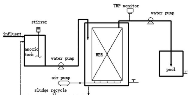
Fig. 1 A process flow diagram of the DMAC wastewater treatment.
