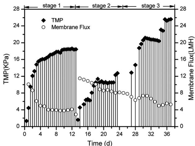
Fig. 3 Transmembrane pressure and membrane flux profile.
