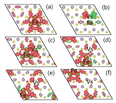
Fig. 5 The spatial distribution of the spin density for (a)  $Mo_{15}FeS_{32}$ , (b)  $Mo_{15}FeS_{31}-A$ , (c)  $Mo_{15}FeS_{31}-B$ , (d)  $Mo_{15}FeS_{31}-C$ , (e)  $Mo_{15}FeS_{31}-D$ , and (f)  $Mo_{15}FeS_{31}-E$ . The S, Mo, and Fe atoms are denoted by yellow, purple, and dark yellow spheres, respectively. The red isosurface corresponds to the spin-up density, and the green one represents the spin-down density.
