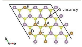
Fig. 1 Top view of the  $4\times4\times1$  supercell of the defective  $1H-MoS_2$  impurities. Five configurations are taken into account in this work and marked as  $Mo_{15}XS_{31}-A$ , B, C, D, or E according to the distance between the dopant and S vacancy.
