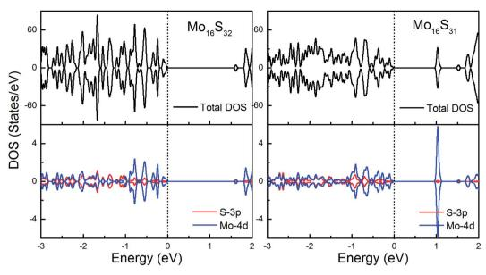
Fig. 6 Total DOS and partial DOS for pristine 1H-MoS<sub>2</sub> with and without S vacancies. The dashed line indicates the Fermi level at 0 eV.
