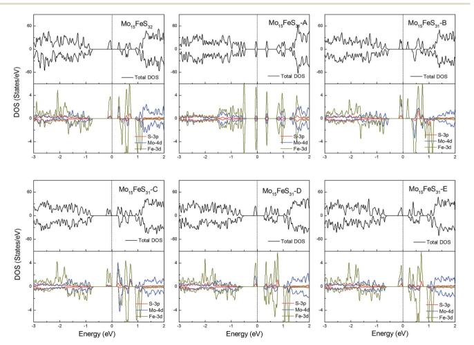
Fig. 7 Total DOS and partial DOS for each atomic species in the all Fe-doped 1H-MoS<sub>2</sub>. The dashed line indicates the Fermi level at 0 eV.
