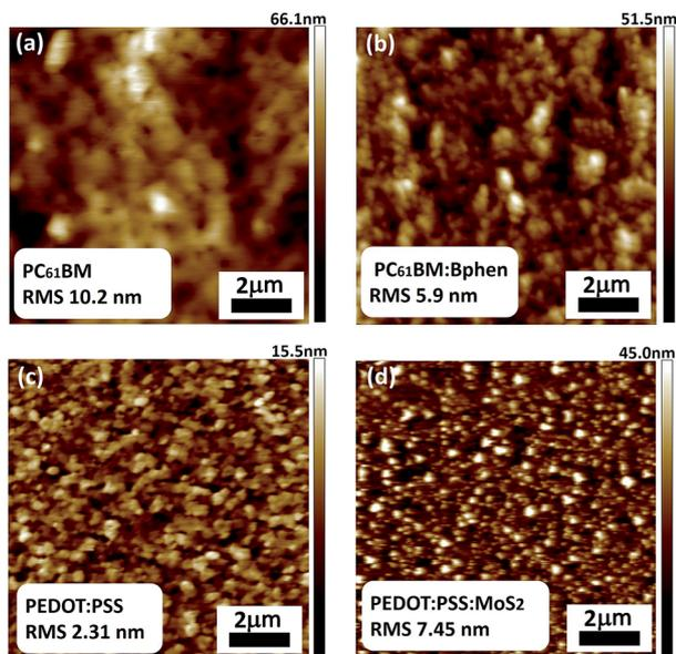
Fig. 5 AFM topographic images of films of (a) PC<sub>61</sub>BM, (b) PC<sub>61</sub>-BM:Bphen (0.5 wt%), (c) PEDOT:PSS, and (d) PEDOT:PSS:MoS<sub>2</sub> (0.1 wt%).
