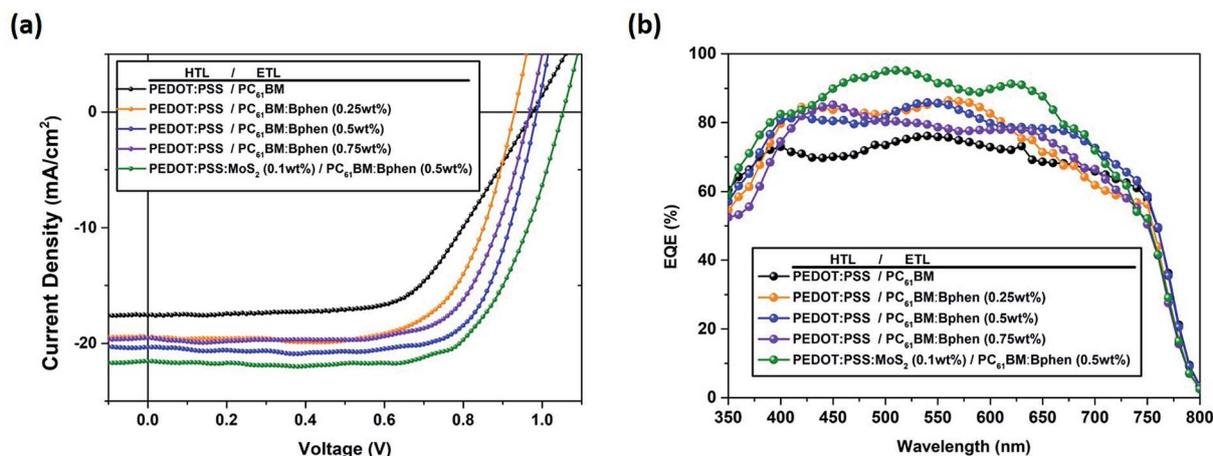
Fig. 2 (a)  $J$ - $V$  characteristics of perovskite devices incorporating Bphen at various contents (0, 0.25, 0.5, 0.75 wt%) in the ETL and incorporating MoS<sub>2</sub> (0.1 wt%) in PEDOT:PSS as the HTL, based on ETL containing 0.5 wt% Bphen, measured under standard 1 sun AM 1.5G simulated solar irradiation. (b) EQE spectra of perovskite devices.
