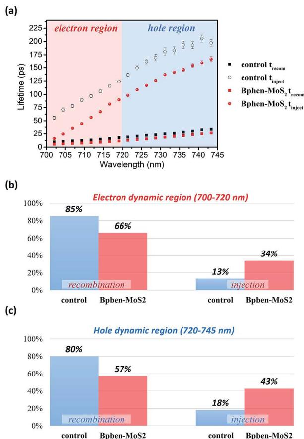
Fig. 8 (a) Wavelength-dependent lifetimes extracted from the values of  $\Delta A$ . Average percentages for the decomposed relaxation processes in the two different regions: (b) 700–720 nm for electrons and (c) 720–745 nm for holes.
