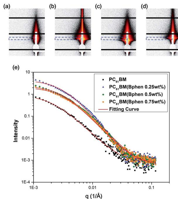
Fig. 6 (a–d) 2-D GISAXS patterns of PC<sub>61</sub>BM films containing (a) 0, (b) 0.25, (c) 0.5, and (d) 0.75 wt% Bphen; blue lines represent integral areas. (e) GISAXS profiles of perovskite/PC<sub>61</sub>BM films containing various weight fractions of Bphen. All profiles were fitted using calculated model intensities (solid lines).
