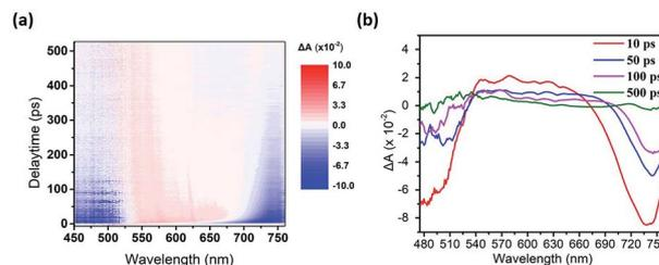
Fig. 7 (a) 2-D Plot of the ultrafast transient absorption difference ( $\Delta A$ ) on the structure: ITO/PEDOT:PSS:MoS<sub>2</sub> (0.1 wt%)/CH<sub>3</sub>NH<sub>3</sub>PbI<sub>3-x</sub>Cl<sub>x</sub>/PC<sub>61</sub>BM:Bphen (0.5 wt%). (b) Transient absorption spectra at various time delays.
