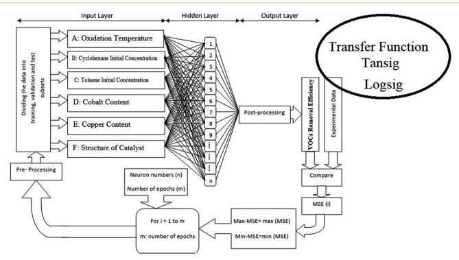
Fig. 1 ANN structure and related flowchart used in this study.
