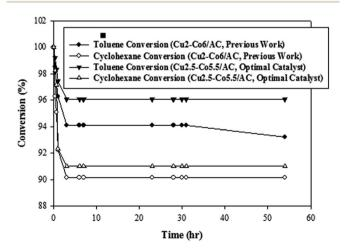
Fig. 11 Long performance of Cu2.5-Co5.5/AC (optimal catalyst) and Cu2-Co6/AC (pervious work) for simultaneous conversion of toluene and cyclohexane in air (initial concentration = 1000 ppmv and oxidation temperature = 250 °C).
