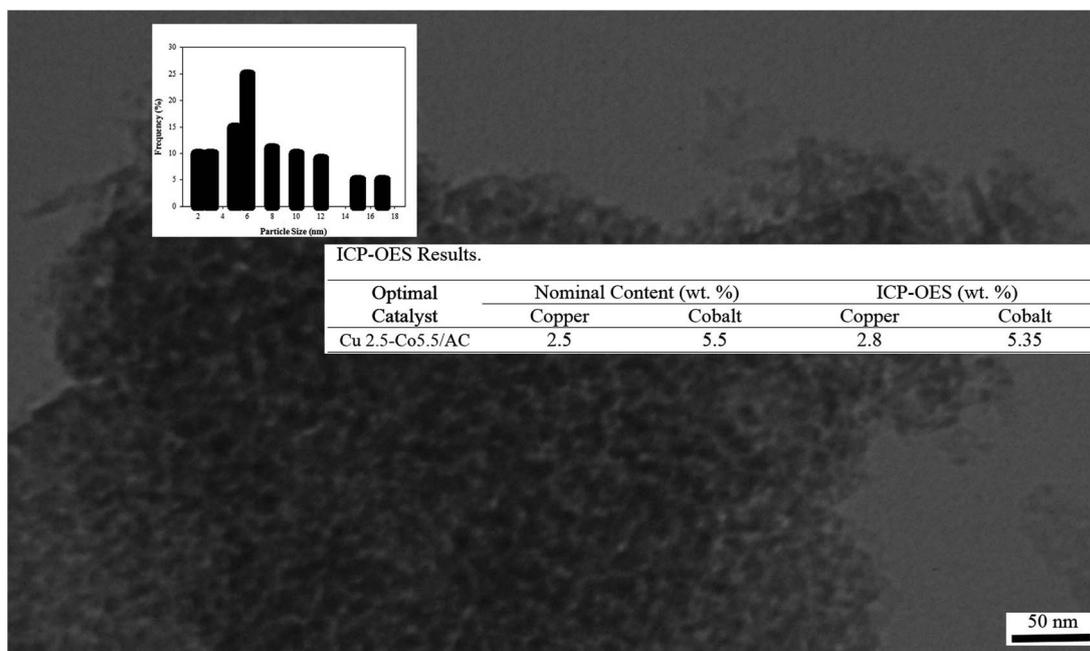
Fig. 9 TEM and ICP results of Cu<sub>2.5</sub>–Co<sub>5.5</sub>/AC as an optimal catalyst.
