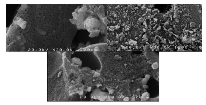
Fig. 10 FESEM results of Cu2.5-Co5.5/AC as an optimal catalyst.
