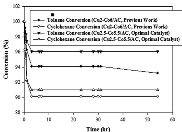
Fig. 11 Long performance of Cu<sub>2.5</sub>-Co<sub>5.5</sub>/AC (optimal catalyst) and Cu<sub>2</sub>-Co<sub>6</sub>/AC (previous work) for simultaneous conversion of toluene and cyclohexane in air (initial concentration = 1000 ppmv and oxidation temperature = 250 °C).
