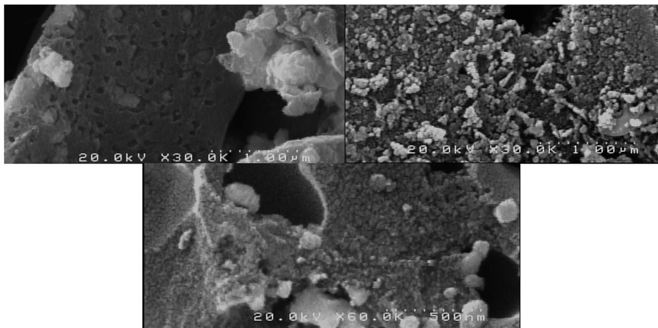
Fig. 10 FESEM results of Cu<sub>2.5</sub>-Co<sub>5.5</sub>/AC as an optimal catalyst.
