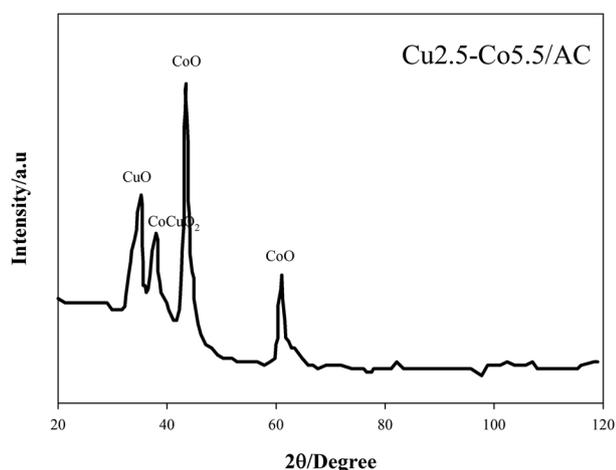
Fig. 8 XRD results of Cu<sub>2.5</sub>–Co<sub>5.5</sub>/AC as an optimal catalyst.
