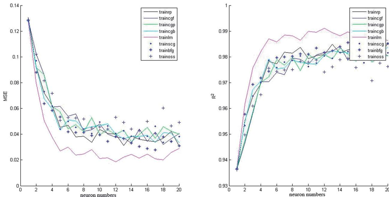
Fig. 4 Effect of the number of neurons on MSE and correlation coefficient ( $R^2$ ) values for various training algorithms (logsig function in the hidden layer).
