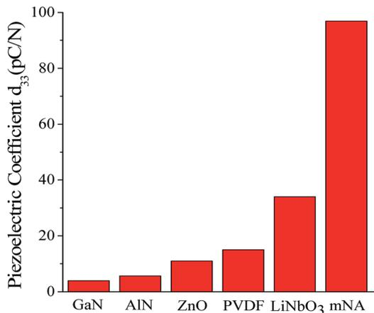
Fig. 2 A visual comparison of  $d_{33}$  of some well-known piezoelectric materials and mNA. The piezoelectric coefficient of GaN,<sup>36</sup> AlN,<sup>7</sup> ZnO,<sup>8</sup> PVDF<sup>14</sup> and LiNbO<sub>3</sub> (ref. 9) were obtained from experiments.
