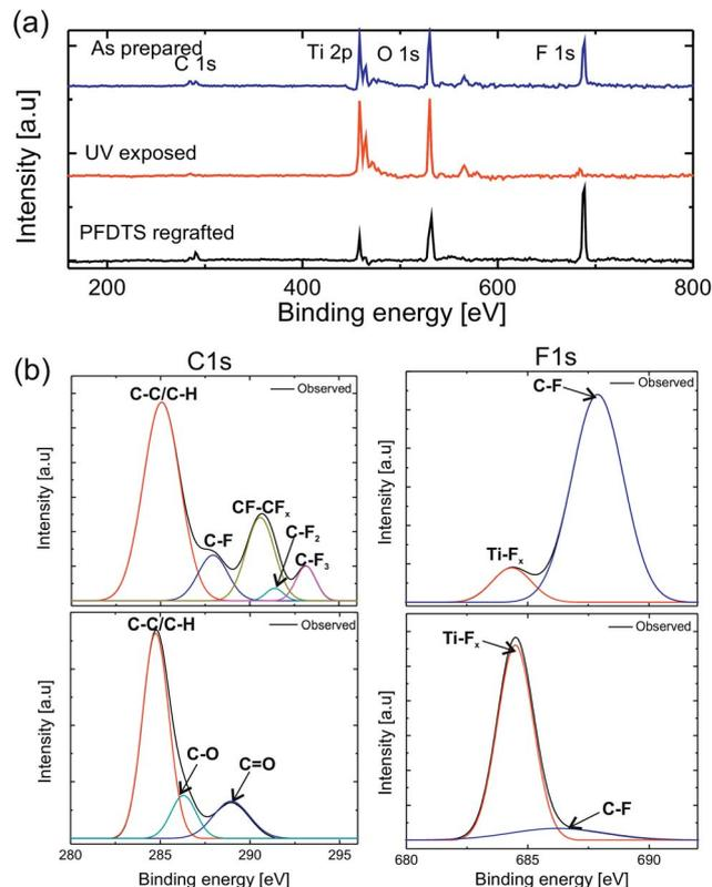
Fig. 5 (a) XPS survey spectra showing the peaks corresponding to different elements present on the surface of as prepared superoleophobic, UV exposed and PFDTs re-grafted surface. (b) The core XPS spectra of C 1s and F 1s of the superoleophobic and UV exposed substrate.
