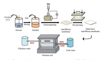
Fig. 1 Schematic diagram of the preparation of PA-6 multi-layer nanofibrous membranes and filtration cell set-up.
