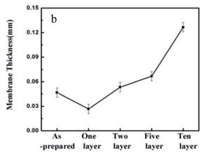
Fig. 2 (a) Photography image of 10 layer nanofibrous membranes. (b) The thickness of nanofibrous membranes as a function of the number of layers.
