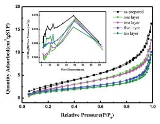
Fig. 4 Nitrogen adsorption—desorption isotherms and pore size distributions of PA-6 nanofibrous membrane with different number of layers.
