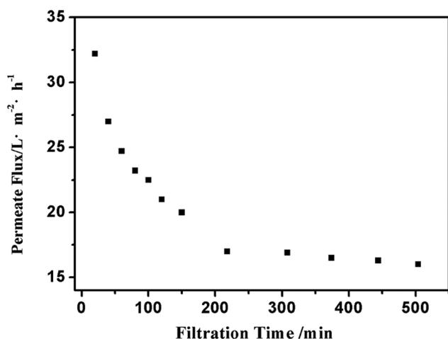
Fig. 8 Permeate flux of 10 layer nanofibrous membranes for removing indigo dye molecules in solution.
