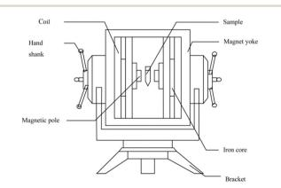
Fig. 1 Schematic of the static magnetic field apparatus.
