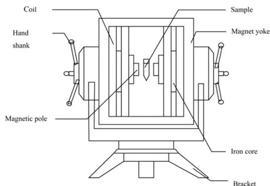
Fig. 1 Schematic of the static magnetic field apparatus.
