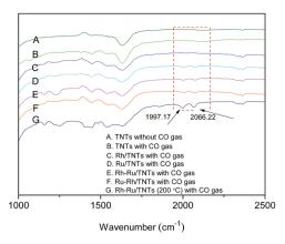
Fig. 5 FT-IR spectra of TNTs without CO gas (A); samples with CO gas: TNTs (B), Rh/TNTs (C), Ru/TNTs (D), Rh-Ru/TNTs (E), Ru-Rh/ TNTs (F), Rh-Ru/TNTs (200 °C) (G),
