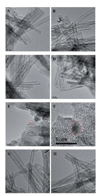
Fig. 3 TEM images of Rh/TNTs (A), Ru/TNTs (B), Rh–Ru/TNTs (C), Ru–Rh/TNTs (D), Rh–Ru/TNTs (200  $^{\circ}$ C) (E), and HRTEM image of the selected area of E (F), Rh–Ru/TNTs-U1 (G), Rh–Ru/TNTs-U2 (H).
