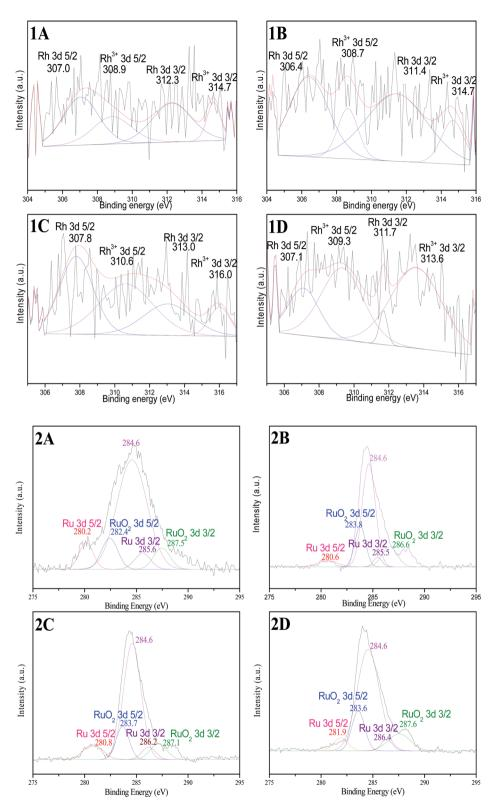
Fig. 4 High-resolution XPS spectra of Rh 3d in Rh/TNTs (1A), Rh-Ru/TNTs (1B), Ru-Rh/TNTs (1C), Rh-Ru/TNTs (200  $^{\circ}$ C) (1D), and Ru 3d in Ru/TNTs (2A), Rh-Ru/TNTs (2B), Ru-Rh/TNTs (2C), Rh-Ru/TNTs (200  $^{\circ}$ C) (2D).
