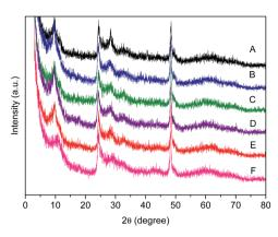
Fig. 1 XRD patterns of TNTs (A), Rh/TNTs (B), Ru/TNTs (C), Rh-Ru/TNTs (D), Ru-Rh/TNTs (E), Rh-Ru/TNTs (200 °C) (F).
