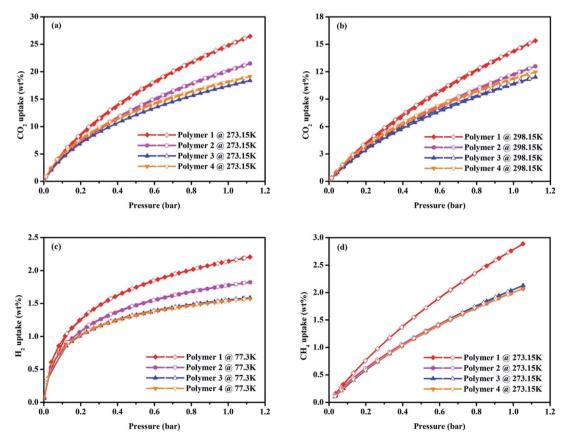
Fig. 4 Volumetric  $CO_2$  adsorption isotherms and desorption isotherms up to 1.13 bar at 273.15 K (a), volumetric  $CO_2$  adsorption isotherms and desorption isotherms up to 1.13 bar at 298.15 K (b), volumetric  $H_2$  adsorption isotherms and desorption isotherms up to 1.13 bar at 77.3 K (c) and volumetric  $CH_4$  adsorption isotherms and desorption isotherms up to 1.13 bar at 273.15 K (d) of all the samples.
