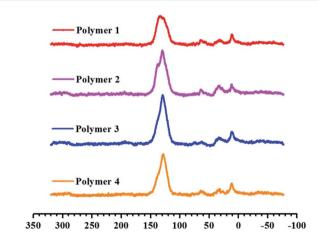
Fig. 1 Cross-polarization (CP)  $^{13}$ C MAS natural abundance NMR spectra of materials from Polymer 1 to Polymer 4.
