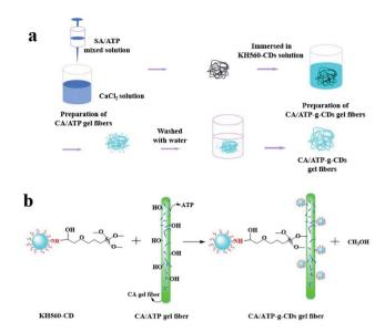
Scheme 2 Schematic of preparation of CA/ATP-g-CDs gel fibers and the surface grafting of CA/ATP gel fibers by KH560-CDs.
