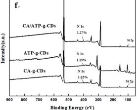
Fig. 3 Fluorescent images and XPS survey scan of CA-g-CDs and ATP-g-CDs.
