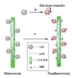
Scheme 3 Schematic illustration of quenching process of CA/ATP-q-CDs gel fibers.
