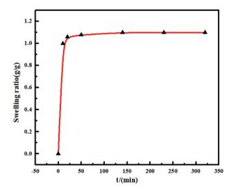
Fig. 4 Swelling ratio of CA/ATP-g-CDs gel fibers.
