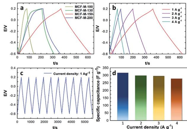
Fig. 6 (a) Charge–discharge profiles of MCF-M-*T* samples at a current density of  $1 \text{ A g}^{-1}$ ; (b) charge–discharge profiles of the MCF-M-150 sample at different current densities; (c) cyclic performance of MCF-M-150; (d) calculated specific capacitance at different current densities of MCF-M-150.
