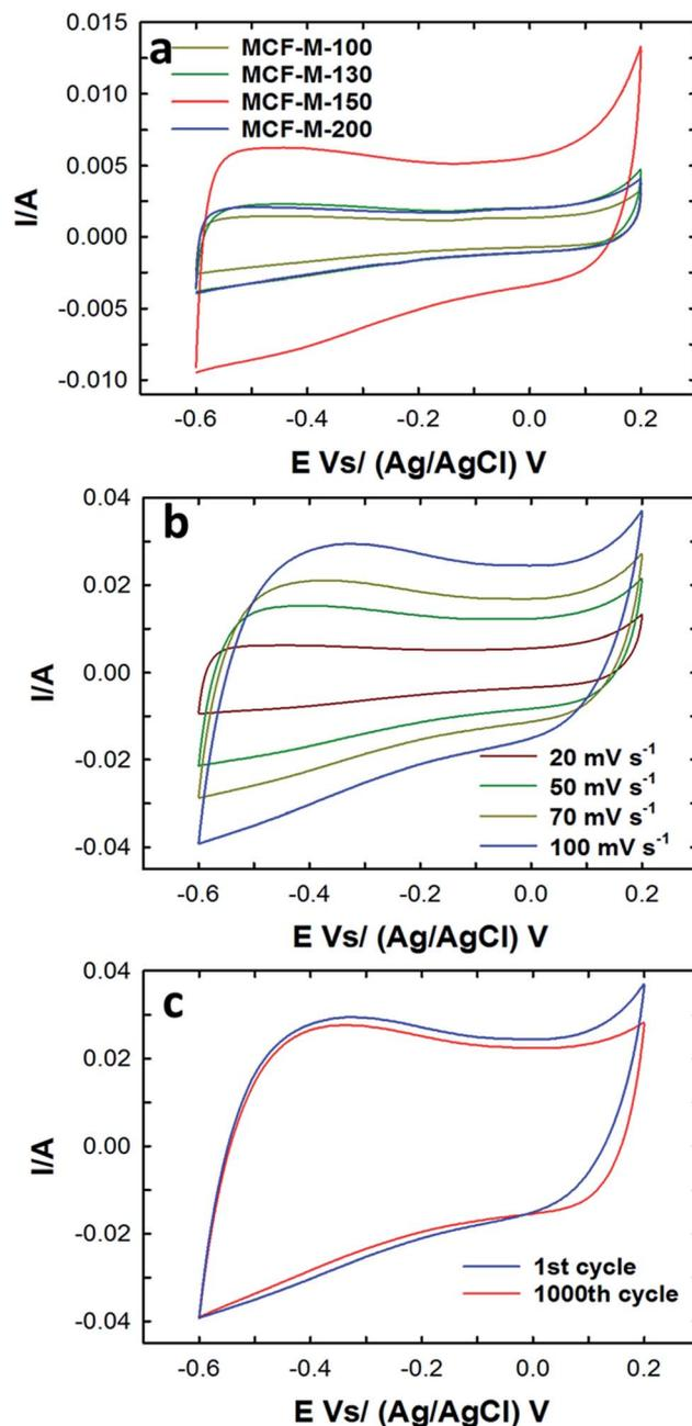
Fig. 5 (a) CV profiles of the MCF-M-*T* samples at a constant scan rate of 20  $\text{mV s}^{-1}$ ; (b) CV profiles of the MCF-M-150 at a different scan rate; (c) CV cyclability of the MCF-M-150 at a constant scan rate of 100  $\text{mV s}^{-1}$ .
