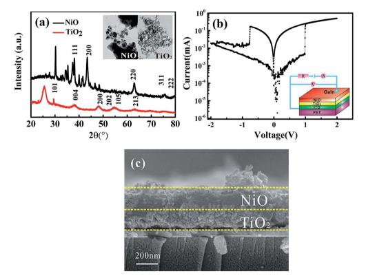
Fig. 1 (a) Typical XRD patterns of the NiO and TiO<sub>2</sub> thin films. The inset shows the TEM images of the as-grown NiO and TiO<sub>2</sub> nanoparticles. (b) I-V characteristics of the Galn/NiO/TiO<sub>2</sub>/ITO structure. (c) Cross-sectional SEM images of the sample.
