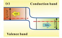
Fig. 5 Energy band diagrams for NiO/TiO<sub>2</sub> in a (a) dynamic equilibrium, (b) forward bias, and (c) reverse bias
