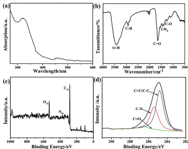
Fig. 2 (a) UV-vis absorption and (b) FT-IR spectra of DMF-CDs; (c) XPS survey of DMF-CDs; (d) XPS fitting of C1s in DMF-CDs.
