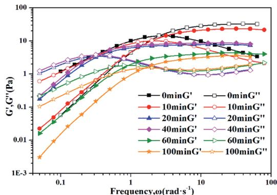
Fig. 6 Dynamic frequency sweep of 30 mM 12-2-12·2Br<sup>-</sup>/10 mM *trans*-OMCA with different UV irradiation time at 25 °C.
