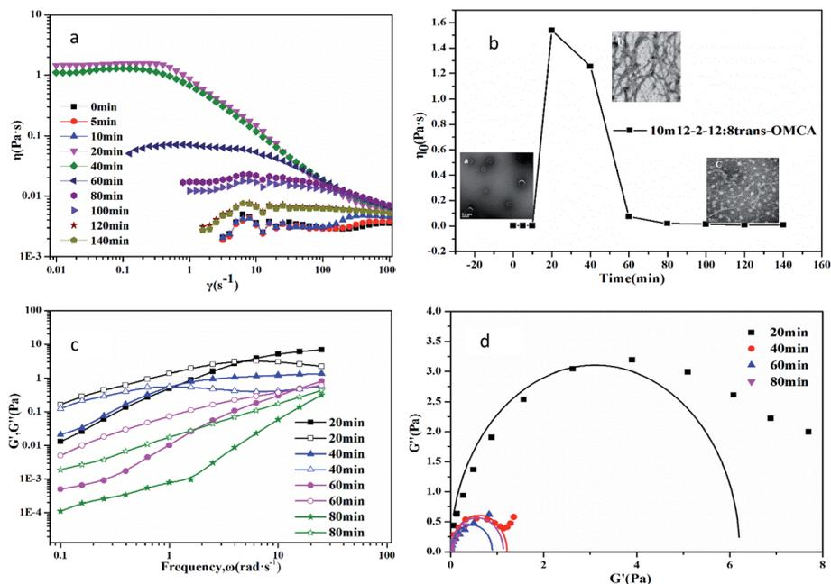
Fig. 7 Photoresponsive viscoelasticity of 10 mM 12-2-12-2Br<sup>-</sup> / 8 mM *trans*-OMCA system at 25 °C; (a) steady shear viscosity, (b) zero-shear viscosity, (c) dynamic frequency sweep, and (d) Cole–Cole plots.
