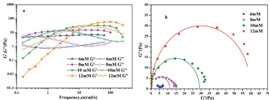
Fig. 3 Dynamic frequency sweep (a) and Cole–Cole plots (b) for 30 mM  $12\text{-}2\text{-}12\cdot 2\text{Br}^-$  with different concentrations of *trans*-OMCA (6 mM, 8 mM, 10 mM, and 12 mM) at 25 °C ( $G'$ : elastic modulus;  $G''$ : viscous modulus).
