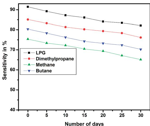
Fig. 16 Stability of pristine and PEDOT–PSS thin film doped with EG.
