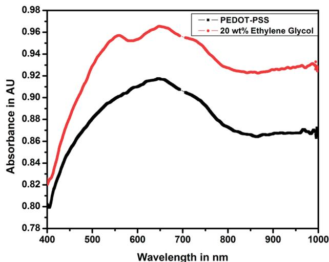
Fig. 7 UV-visible spectra of pristine and PEDOT-PSS thin film doped 20 wt% EG.
