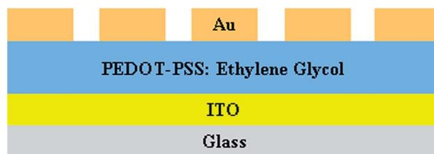
Fig. 3 Schematic representation of the sensor device on ITO-coated glass.
