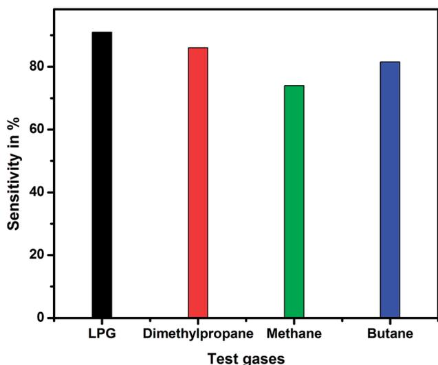
Fig. 17 Selectivity studies for different test gases.
