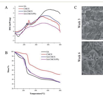
Fig. 3 (A) and (B) DSC and TGA curves of samples. (C) Scanning electron microscopy images of degradation of SA/CMCS and SA/CMCS/PPy hydrogel.
