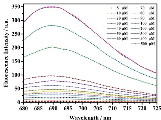
Fig. 5 Fluorescence intensity increase of probe **mbac** (10  $\mu\text{M}$ ) upon the addition of  $\text{ClO}^-$  (5–500  $\mu\text{M}$ ),  $\lambda_{\text{ex}} = 660 \text{ nm}$ . The system was PBS (pH = 7.4). The fluorescence intensity was determined at 690 nm.
