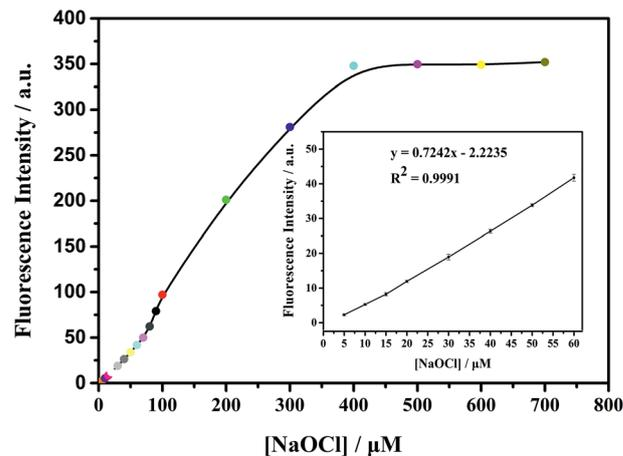
Fig. 3 Fluorescence intensity increases with  $\text{ClO}^-$  concentration ( $\lambda_{\text{ex}} = 660 \text{ nm}$ ). The system contained the probe **mbac** ( $10 \mu\text{M}$ ) in PBS ( $\text{pH} = 7.4$ ). Each data point is the average of three parallel experiments. The inset graphic showing the correlation between the fluorescence response of **mbac** and the concentration of  $\text{ClO}^-$ .
