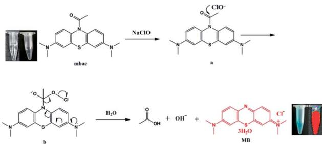
**Scheme 1** Possible mechanism: the cleavage of the amide bond of the fluorescent probe **mbac** results from interacting with  $\text{ClO}^-$ . (The left side of the illustration is the view of the naked eye, and the right side is the view under the Pearl® Impulse Small Animal Imaging System).
