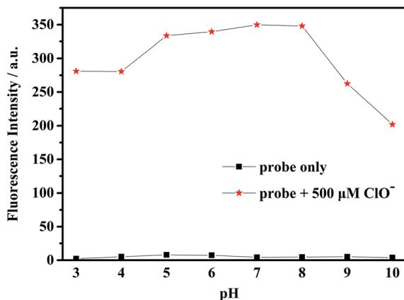
Fig. 2 Fluorescence intensity of the probe **mbac** ( $10 \mu\text{M}$ ) with and without  $\text{ClO}^-$  ( $500 \mu\text{M}$ ) in water at different pH conditions, ( $\lambda_{\text{ex}} = 660 \text{ nm}$ ).
