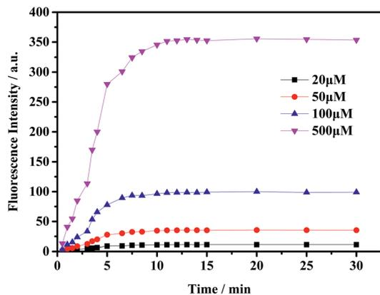
Fig. 1 The time-dependent fluorescence changes ( $\lambda_{\text{ex}} = 660 \text{ nm}$ ) acquired from a mixture of the probe **mbac** ( $10 \mu\text{M}$ ) and  $\text{ClO}^-$  ( $20 \mu\text{M}$ ,  $50 \mu\text{M}$ ,  $100 \mu\text{M}$  and  $500 \mu\text{M}$ ) in PBS ( $\text{pH} = 7.4$ ) solution at room temperature. Data represent the average of three parallel experiments.
