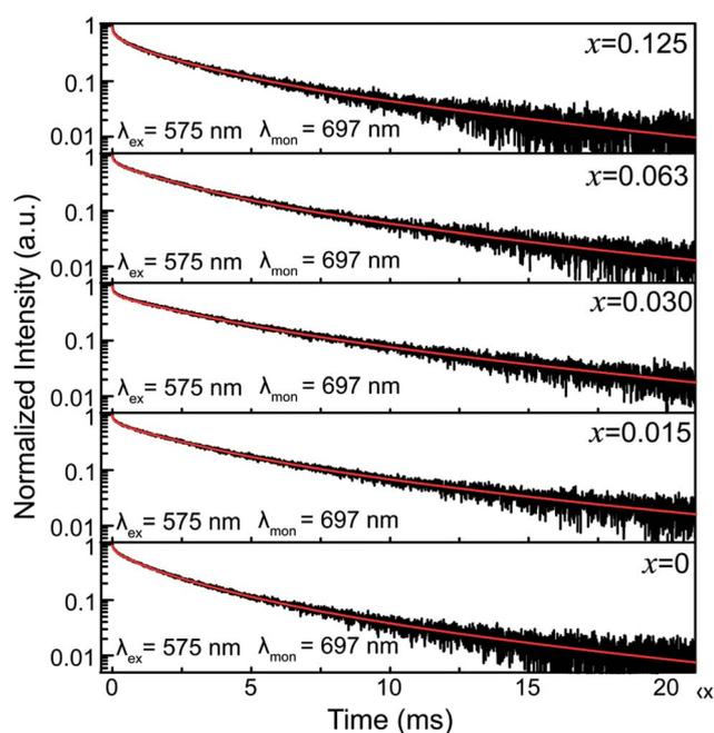
Fig. 9 The decay curves of  $\text{ZGGO}:\text{Cr}^{3+}$  nanoparticles with various  $\text{Sn}^{4+}$  concentrations ( $x = 0, 0.015, 0.030, 0.063$  and  $0.125$ ) monitored at 697 nm under 575 nm excitation.
