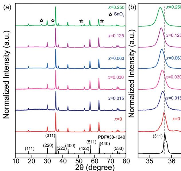
Fig. 1 (a) XRD patterns of ZGGSO: $\text{Cr}^{3+}$  powders with various  $\text{Sn}^{4+}$  concentrations ( $x = 0, 0.015, 0.030, 0.063, 0.125$  and  $0.250$ ). (b) The (311) peak position as a function of  $\text{Sn}^{4+}$  substitution concentration.
