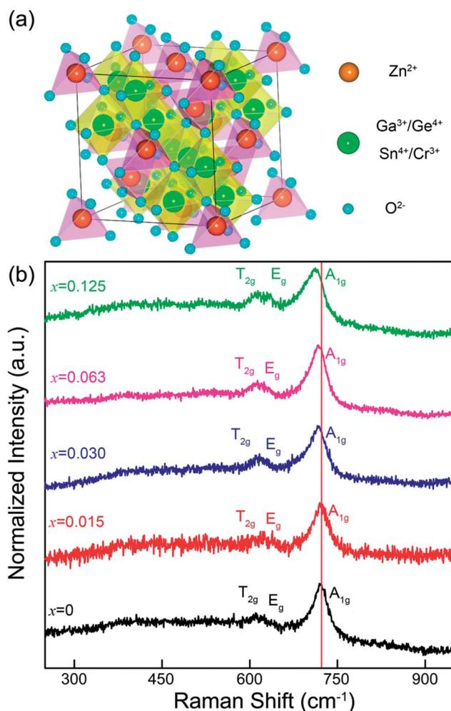
**Fig. 4** (a) A cell of ZnGa<sub>2</sub>O<sub>4</sub> with a spinel structure (AB<sub>2</sub>X<sub>4</sub> formula). (b) Raman spectra of ZGGSO:Cr<sup>3+</sup> nanoparticles with different Sn<sup>4+</sup> substitution concentrations ( $x = 0, 0.015, 0.030, 0.063$  and  $0.125$ ).
