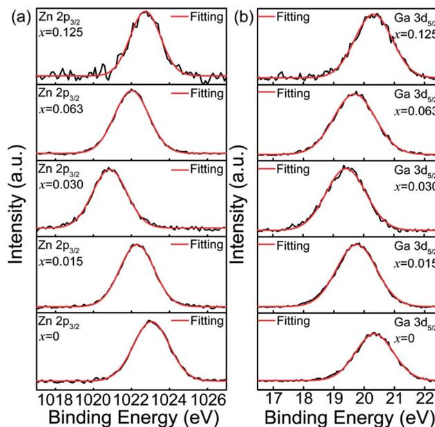
Fig. 8 XPS spectra of (a) Zn  $2p_{3/2}$  and (b) Ga  $3d_{5/2}$  core levels for ZGGSO: $\text{Cr}^{3+}$  nanoparticles with various  $\text{Sn}^{4+}$  concentrations ( $x = 0, 0.015, 0.030, 0.063$  and  $0.125$ ).
