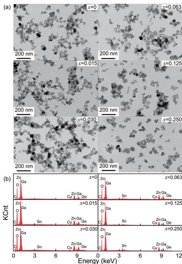
**Fig. 2** (a) TEM images and (b) EDS of ZGGSO:Cr<sup>3+</sup> nanoparticles with various Sn<sup>4+</sup> concentrations ( $x = 0, 0.015, 0.030, 0.063, 0.125$  and  $0.250$ ).
