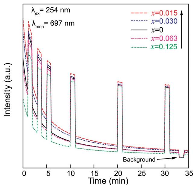
Fig. 11 PSL spectra of ZGGSO: $\text{Cr}^{3+}$  nanoparticles with various  $\text{Sn}^{4+}$  concentrations monitored at 697 nm (stimulation wavelength: 808 nm) after the stoppage of 254 nm irradiation.
