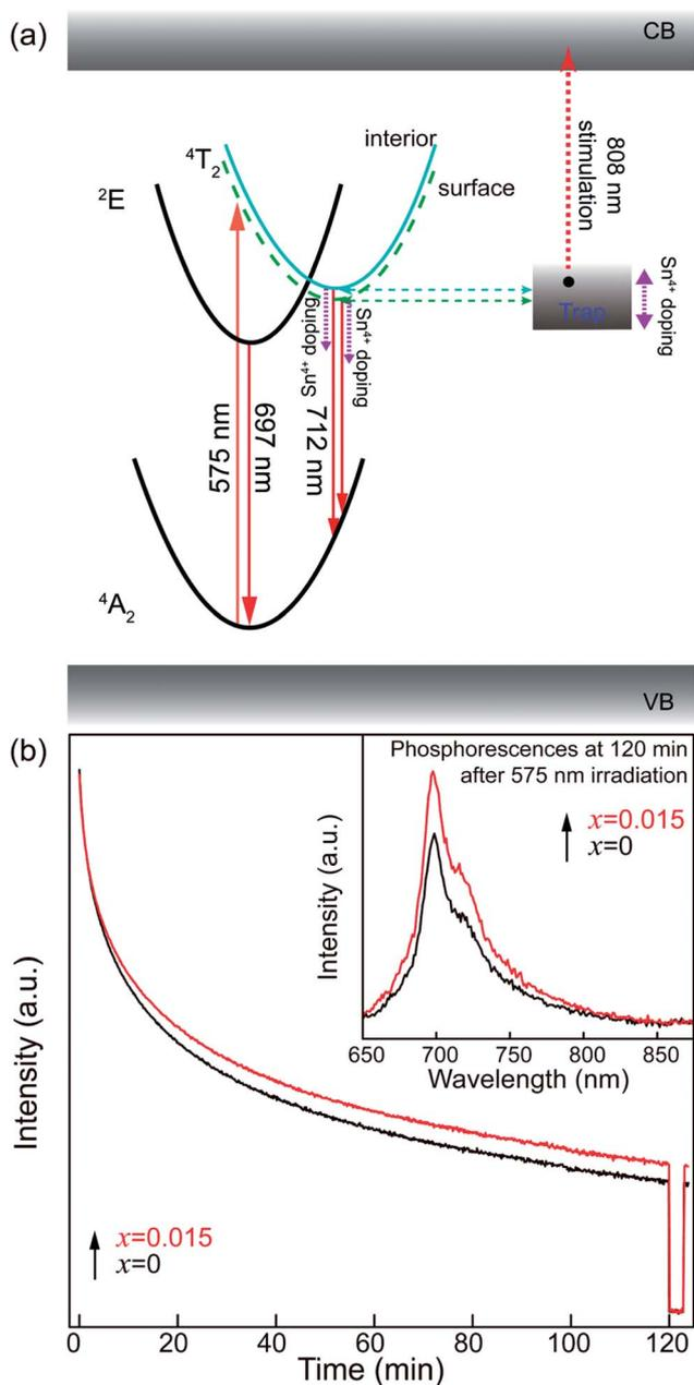
Fig. 10 (a) A schematic configuration coordinate diagram related to the energy transfer from  $\text{Cr}^{3+}$  ion to the deep traps under the  ${}^4\text{A}_2$ – ${}^4\text{T}_2$  excitation. (b) The afterglow decay curves of ZGGSO: $\text{Cr}^{3+}$  nanoparticles without and containing  $\text{Sn}^{4+}$  ( $x = 0, 0.015$ ) upon 575 nm excitation. The inset shows their phosphorescence spectra.
