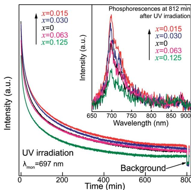
Fig. 6 The afterglow decay curves of ZGGSO:Cr<sup>3+</sup> nanoparticles with various Sn<sup>4+</sup> substitution concentrations ( $x = 0, 0.015, 0.030, 0.063$  and  $0.125$ ) upon 254 nm excitation. The inset shows their phosphorescence spectra.
