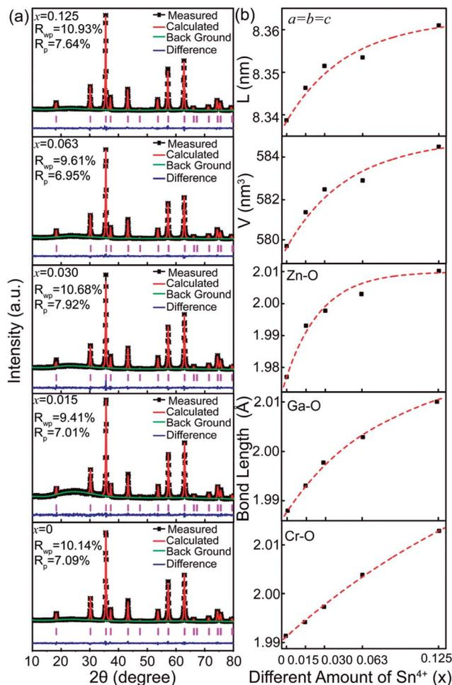
**Fig. 3** (a) The Rietveld refinements of XRD data for ZGGSO:Cr<sup>3+</sup> nanoparticles with various Sn<sup>4+</sup> concentrations ( $x = 0, 0.015, 0.030, 0.063, 0.125$  and  $0.250$ ). (b) The calculated lattice constant, cell volume and Zn–O, Ga–O and Cr–O bond lengths as a function of Sn<sup>4+</sup> substitution concentration.
