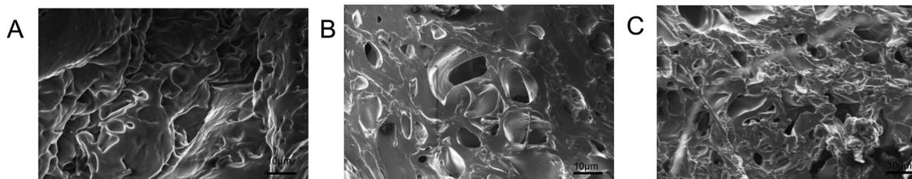
Fig. 3 The SEM image of hydrogels: PM (A), PMA-1 (B) and PMA-2 (C). All the samples were prepared by saturated swelling and freeze-dried.
