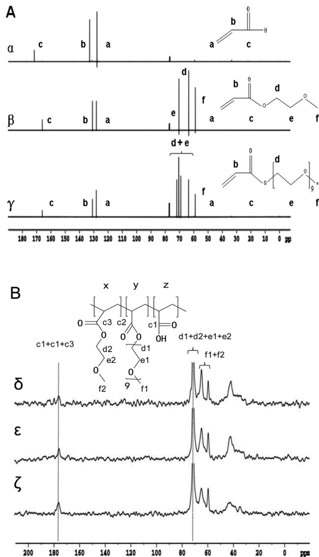
Fig. 2 (A)  $^{13}\text{C}$  NMR spectra in  $\text{CDCl}_3$  (700 MHz) of AA ( $\alpha$ ), MEA ( $\beta$ ), PEGA ( $\gamma$ ). (B)  $^{13}\text{C}$  CP/MAS NMR spectra (300 MHz) of PM ( $\delta$ ), PMA-1 ( $\epsilon$ ), and PMA-2 ( $\zeta$ ).
