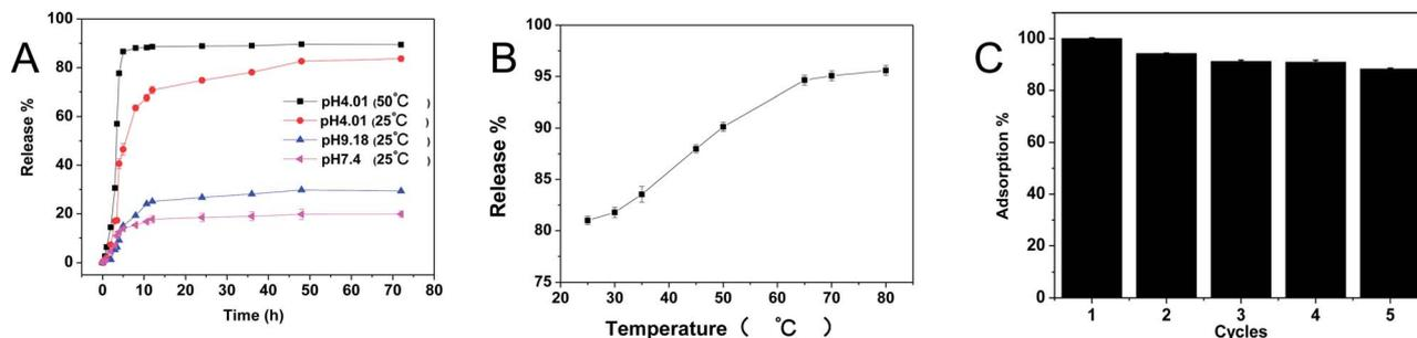
Fig. 10 (A) Time dependence of SBC release from PMA-2 hydrogels in PBS solution (pH = 4.01, 7.4, 9.18) at different temperature. (B) Effect of temperature on release. (C) The regeneration of PMA-2 on brilliant green during five cycles (pH 4.01 PBS solution and 50 °C).
