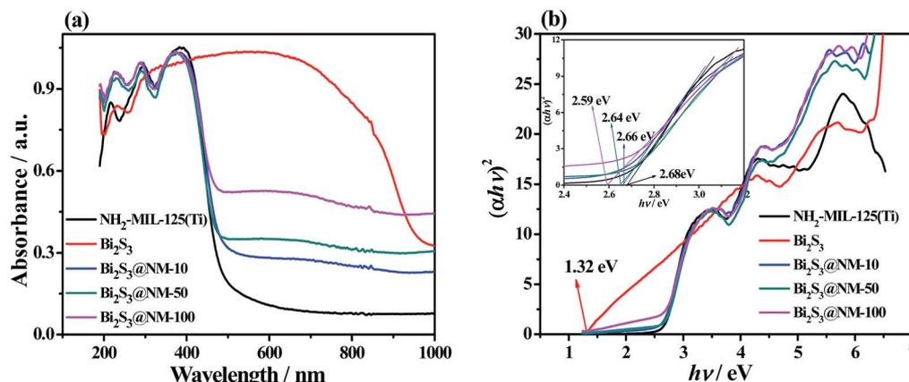
Fig. 4 (a) UV-Vis DRS and (b) the plots of  $(\alpha h\nu)^2$  versus energy ( $h\nu$ ) of the  $\text{NH}_2\text{-MIL-125(Ti)}$ ,  $\text{Bi}_2\text{S}_3$ ,  $\text{Bi}_2\text{S}_3\text{@NM-10}$ ,  $\text{Bi}_2\text{S}_3\text{@NM-50}$ , and  $\text{Bi}_2\text{S}_3\text{@NM-100}$  (the inset: zoomed-in plots of the samples).
