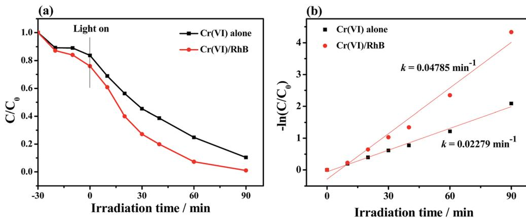
Fig. 8 Photocatalytic reduction (a) and reduction kinetics of Cr(vi) (b) with and without RhB using  $\text{Bi}_2\text{S}_3$ @NM-100 sample (initial concentrations of Cr(vi):  $10 \text{ mg L}^{-1}$  and RhB:  $5 \text{ mg L}^{-1}$ , photocatalyst dosage:  $200 \text{ mg L}^{-1}$ , pH = 3.0).
