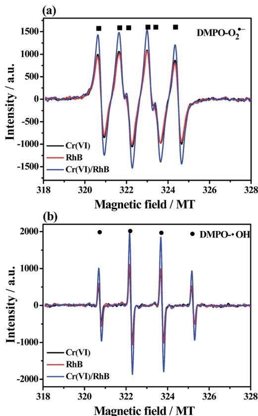
Fig. 12 ESR spectra of (a)  $\text{DMPO-O}_2^{\bullet-}$  and (b)  $\text{DMPO-}\cdot\text{OH}$  formed over  $\text{Bi}_2\text{S}_3@ \text{NH}_2\text{-MIL-125(Ti)}$  in  $\text{Cr(VI)}$ , RhB, and  $\text{Cr(VI)/RhB}$  coexistence systems under visible light ( $\lambda > 420 \text{ nm}$ ) for 10 min.
