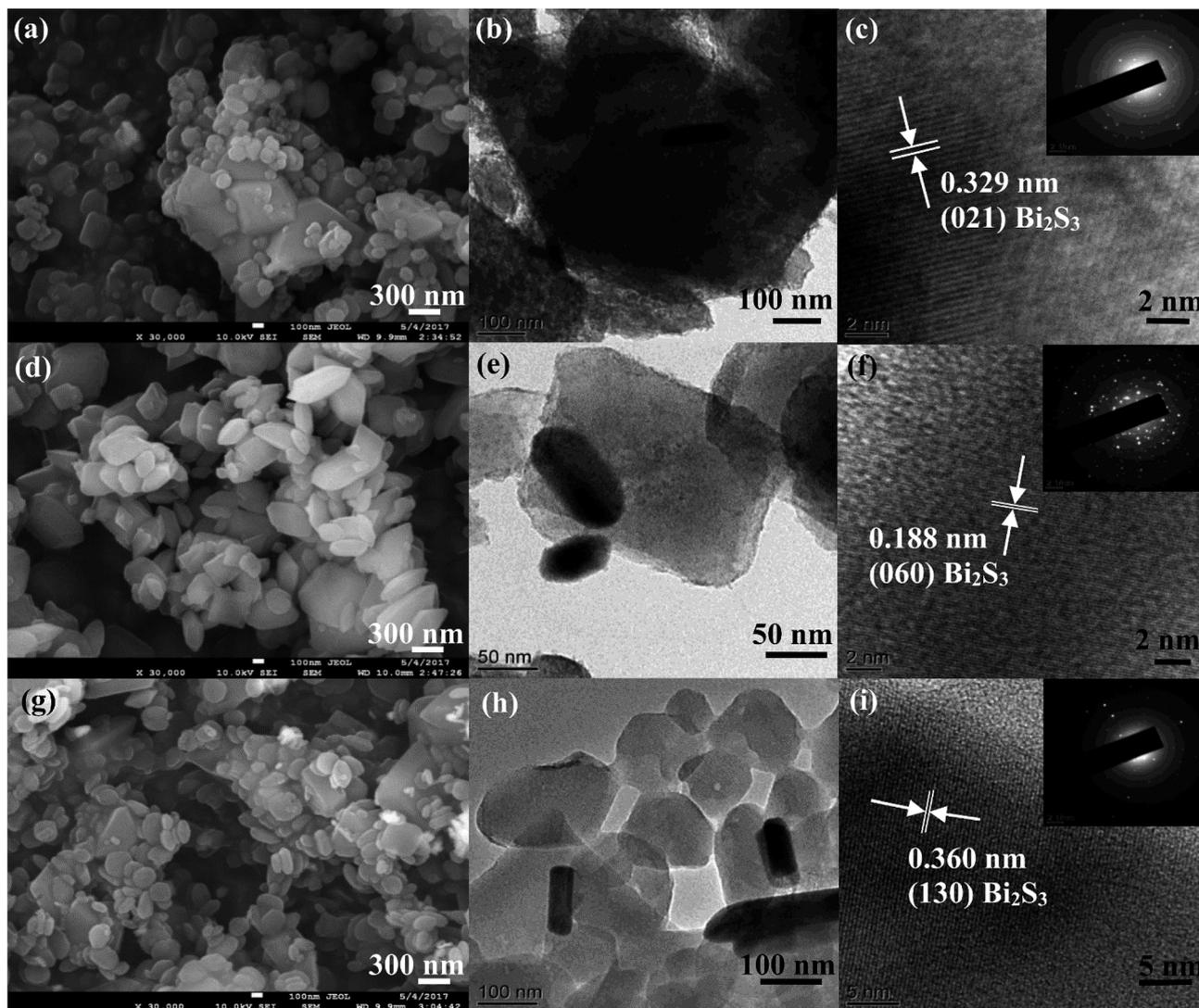
Fig. 3 FE-SEM, TEM and HR-TEM images of (a–c)  $\text{Bi}_2\text{S}_3\text{@NM-10}$ , (d–f)  $\text{Bi}_2\text{S}_3\text{@NM-50}$ , and (g–i)  $\text{Bi}_2\text{S}_3\text{@NM-100}$  nanocomposites, respectively. The insets in (c), (f), and (i) are the corresponding SAED patterns.
