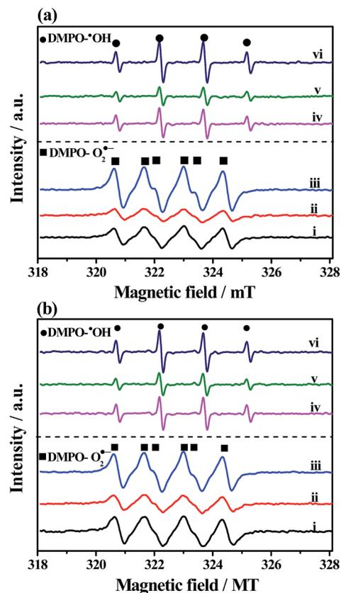
Fig. 11 ESR spectra of DMPO-O<sub>2</sub><sup>•-</sup> and DMPO-•OH in (a) Cr(vi) and (b) RhB solution under visible light ( $\lambda > 420$  nm) for 10 min, including (i) and (iv) for NH<sub>2</sub>-MIL-125(Ti), (ii) and (v) for Bi<sub>2</sub>S<sub>3</sub>, (iii) and (vi) for Bi<sub>2</sub>S<sub>3</sub>@NM-100.
