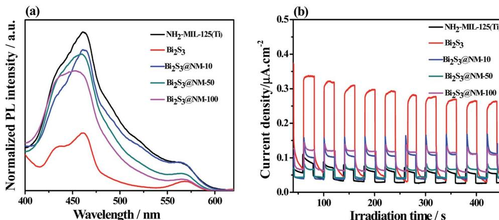
Fig. 5 (a) Photoluminescence spectra ( $\lambda_{\text{ex}} = 350 \text{ nm}$ ) and (b) photocurrent responses of the  $\text{NH}_2\text{-MIL-125(Ti)}$ ,  $\text{Bi}_2\text{S}_3$ ,  $\text{Bi}_2\text{S}_3\text{@NM-10}$ ,  $\text{Bi}_2\text{S}_3\text{@NM-50}$ , and  $\text{Bi}_2\text{S}_3\text{@NM-100}$  nanocomposites.
