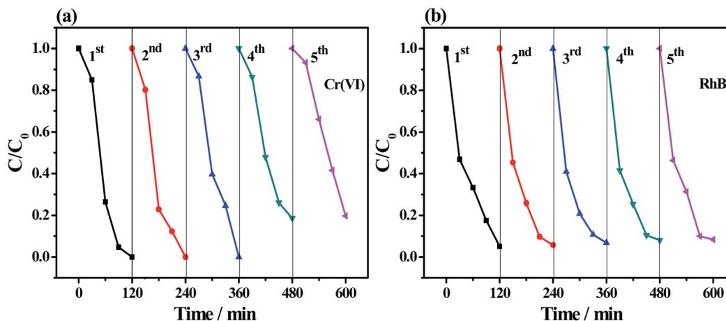
Fig. 9 Recycled test of  $\text{Bi}_2\text{S}_3$ @NM-100 for (a) photocatalytic reduction of Cr(vi) (initial concentration:  $10 \text{ mg L}^{-1}$ , photocatalyst dosage:  $200 \text{ mg L}^{-1}$ , pH = 3.0) and (b) photocatalytic degradation of RhB (initial concentration:  $20 \text{ mg L}^{-1}$ , photocatalyst dosage:  $200 \text{ mg L}^{-1}$ , pH = 7.0).
