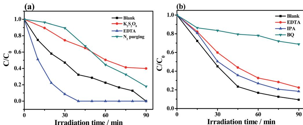
Fig. 10 Photocatalytic activity of the Bi<sub>2</sub>S<sub>3</sub>@NM-100 for (a) Cr(vi) reduction (initial concentration: 20 mg L<sup>-1</sup> photocatalyst dosage: 200 mg L<sup>-1</sup>, pH = 3.0) and (b) RhB degradation (initial concentration: 10 mg L<sup>-1</sup>, photocatalyst dosage: 200 mg L<sup>-1</sup>, pH = 7.0) with different scavengers under light irradiation.
