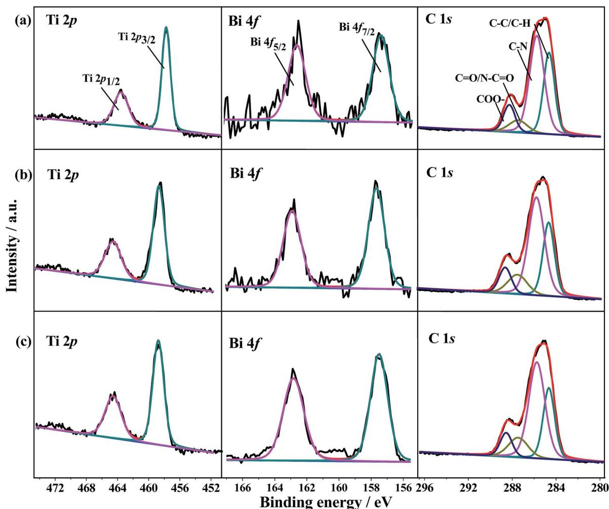
Fig. 2 Ti 2p, Bi 4f, and C 1s high resolution XPS spectra of (a) Bi<sub>2</sub>S<sub>3</sub>@NM-10, (b) Bi<sub>2</sub>S<sub>3</sub>@NM-50, and (c) Bi<sub>2</sub>S<sub>3</sub>@NM-100 nanocomposites.
