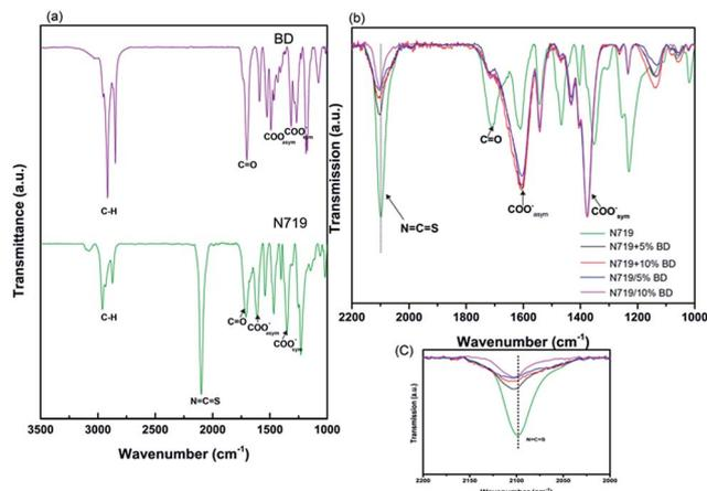
Fig. 4 FTIR Spectra (a) BD and N719 (b) co-sensitized N719 + BD on TiO<sub>2</sub> film and (c) expansion of N=C=S bands.
