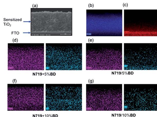
Fig. 6 Cross-sectional image of sensitized TiO<sub>2</sub> (a), EDS mapping images of (b) Ti, (c) Sn, (d) Ru and F of N719 + 5% BD (e) Ru and F of N719/5% BD (f) Ru and F of N719 + 10% BD and (g) Ru and F of N719/10% BD.
