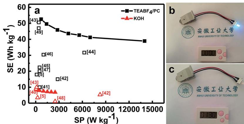
Fig. 9 Ragone plots for the NOC-K based symmetric devices with the TEABF<sub>4</sub>/PC and KOH as the electrolytes (a), and digital images ((b) and (c)) for a light-emitting diode indicator powered by our symmetric cell with the TEABF<sub>4</sub>/PC electrolyte. The red and black data in panel (a) are for aqueous and organic symmetric systems, respectively.
