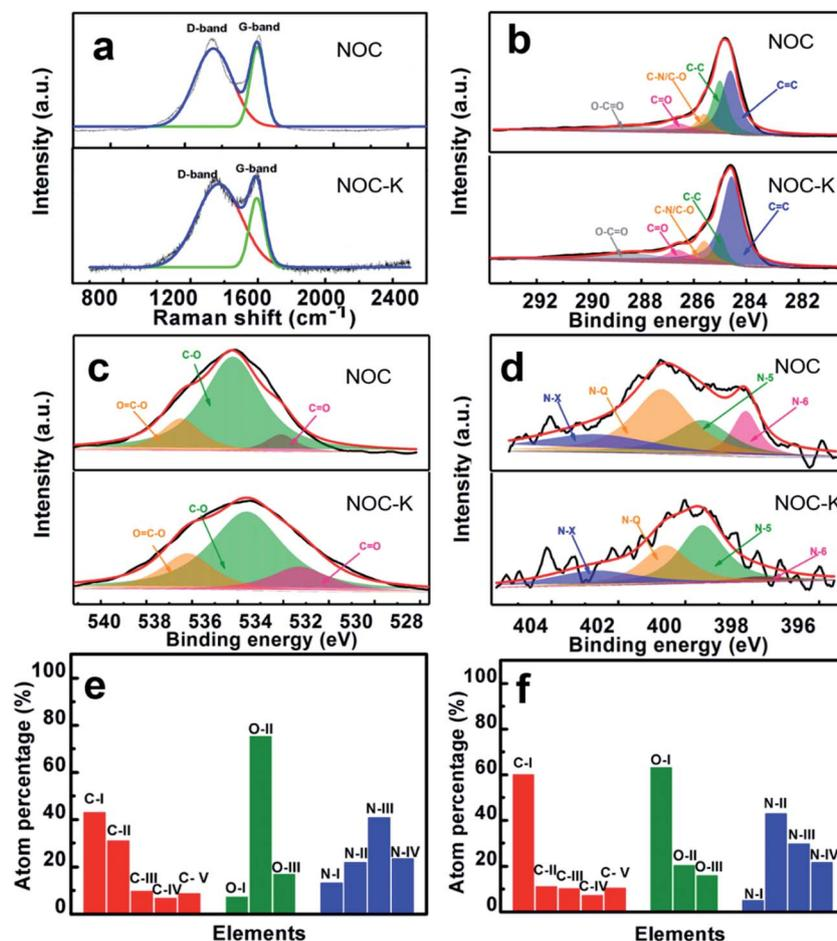
Fig. 4 Raman spectra (a) and high-resolution elemental ((b), C 1s; (c), O 1s; (d), N 1s) XPS spectra and fitted data for the resulting NOC and NOC-K products; Relative content profiles of different types of carbon, nitrogen and oxygen atoms in the NOC (e) and NOC-K (f).
