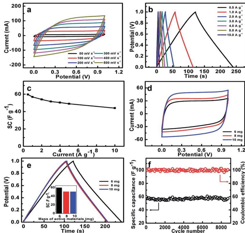
Fig. 7 CV curves (a), CP profiles (b), SC vs. current density (c) for the NOC-K based symmetric device. Typical CV plots ((d),  $100 \text{ mV s}^{-1}$ ) and CP data ((e),  $1 \text{ A g}^{-1}$ ) of the symmetric devices with various loadings of NOC-K as indicated. Cycling behaviors and CE data of the NOC-K based symmetric device (f). The inset in panel (e) for the SCs as a function of total mass loading in one symmetric device.
