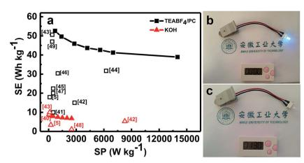
Fig. 9 Ragone plots for the NOC-K based symmetric devices with the TEABF $_4$ /PC and KOH as the electrolytes (a), and digital images ((b) and (c)) for a light-emitting diode indicator powered by our symmetric cell with the TEABF $_4$ /PC electrolyte. The red and black data in panel (a) are for aqueous and organic symmetric systems, respectively.
