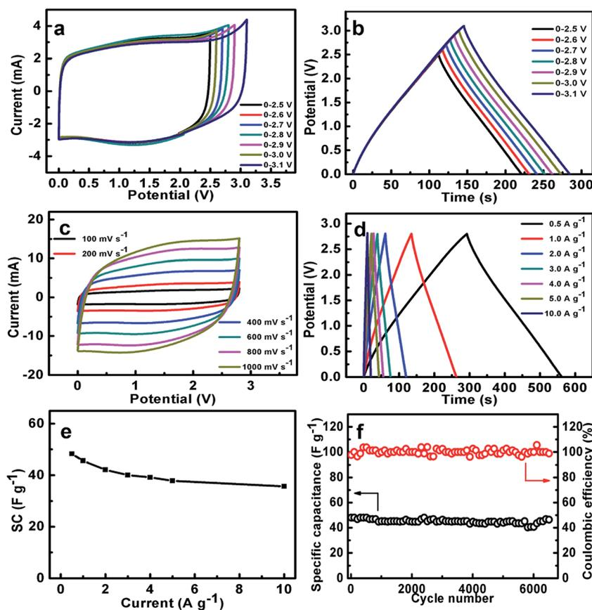
Fig. 8 Electrochemical evaluation of the NOC-K based symmetric device with an aprotic electrolyte of 1 M TEABF<sub>4</sub>/PC: CV curves (a) and CP plots (b) with various upper voltage limits as indicated; CV curves at different sweep rates (c) and CP plots at various current rates (d) within the potential range from 0.0 to 2.8 V; SC as a function of current density (e) and cycling performance ((f),  $0.5 \text{ A g}^{-1}$ ) with the upper potential limit of 2.8 V.
