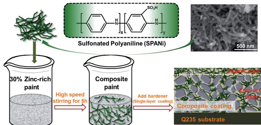
Fig. 1 Structural formula and SEM images of water-soluble SPANi nanofiber and coating preparation of zinc-rich/SPANi composite coating.
