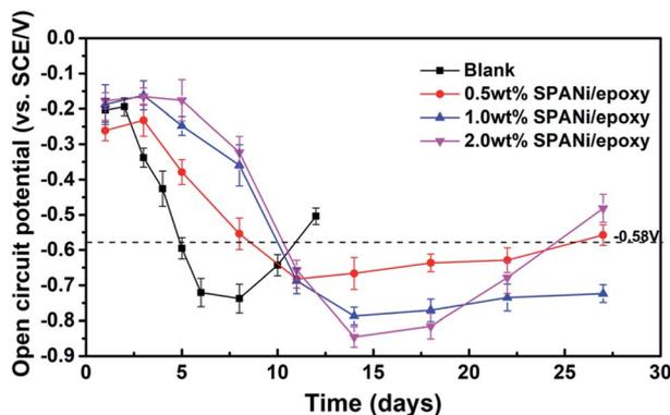
Fig. 3 Open circuit potential for the pure zinc-rich coating, 0.5 wt%, 1.0 wt% and 2.0 wt% SPANi zinc-rich coatings after different immersion times in 3.5 wt% NaCl solution.
