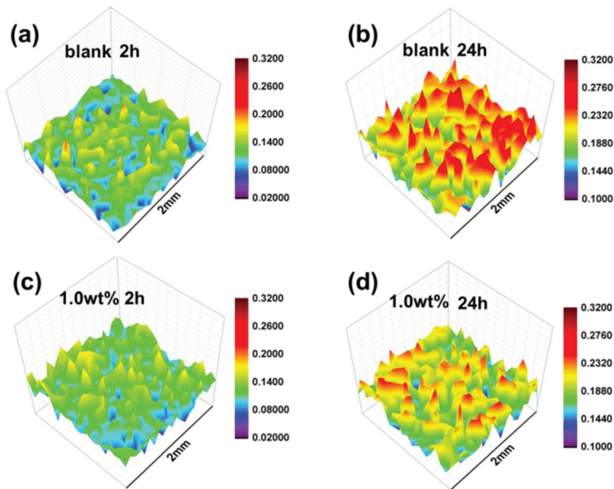
Fig. 9 SVET 3D current density distribution maps of coated steel immersed in 3.5 wt% NaCl solution for 2 h and 24 h. Blank sample: (a), 2 h and (b), 24 h; 1.0 wt% of SPANi zinc-rich coating sample: (c), 2 h and (d), 24 h; unit of current density =  $\mu\text{A cm}^{-2}$ .
