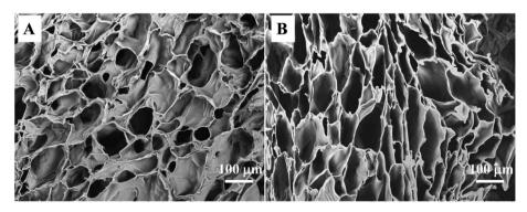
Fig. 2 SEM images of the CTS hydrogel (A) and CC hydrogel (B).
