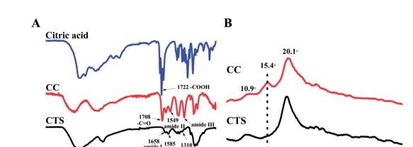
Fig. 1 FTIR spectra (A) and XRD (B) of citric acid, CTS and CC
