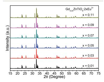
Fig. 1 XRD patterns of the  $Gd_{2-2x}ZnTiO_6:2xEu^{3+}$  (x = 0.01, 0.03, 0.05,0.07, 0.09, and 0.11) phosphors in the  $2\theta$  range of  $15-75^{\circ}$ .
