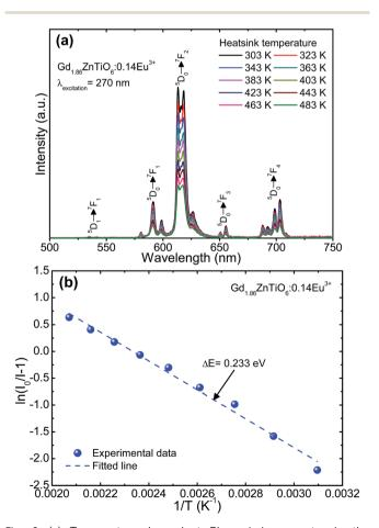
Fig. 6 (a) Temperature-dependent PL emission spectra in the temperature range of 303-483 K with an interval of 20 K and (b) plot of  $ln(I_0/I - 1)$  versus 1/T of the  $Gd_{1.86}ZnTiO_6:0.14Eu^{3+}$  phosphor.
