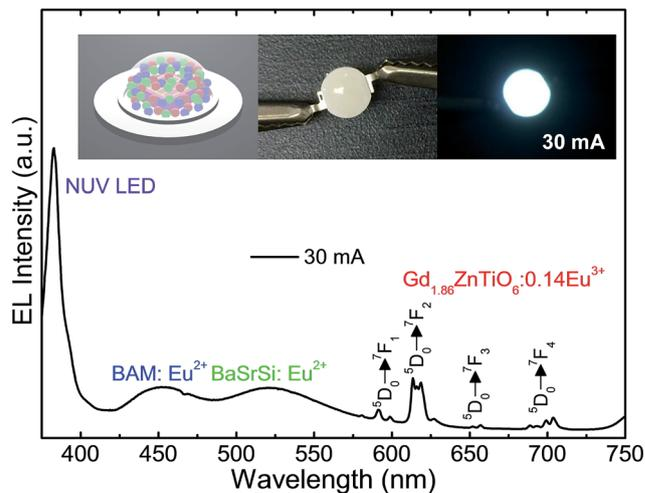
Fig. 9 EL spectrum of the WLED fabricated by the combination of UV LED ( $\lambda \sim 385$  nm), commercial blue-emitting and green-emitting phosphors, and  $\text{Gd}_{1.86}\text{ZnTiO}_6:0.14\text{Eu}^{3+}$  red-emitting phosphor at the injection current of 30 mA under continuous-wave mode. The schematic illustration of WLED and its photographs before/after the current injection were demonstrated in the inset.
