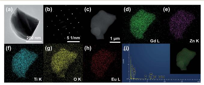
Fig. 3 (a) TEM image, (b) SAED pattern, (c) SEM image, (d-h) elemental mapping images, and (i) EDX spectrum of the Gd<sub>1.86</sub>ZnTiO<sub>6</sub>:0.14Eu<sup>3+</sup> phosphor.
