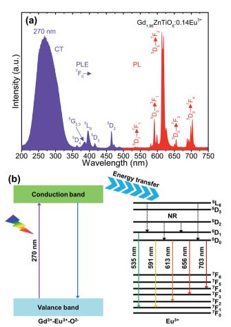
Fig. 4 (a) PLE and PL emission spectra of the  ${\rm Gd_{1.86}ZnTiO_6:0.14Eu^{3+}}$  phosphor and (b) energy level diagram of the  ${\rm Gd_2ZnTiO_6}$  host material and  ${\rm Eu^{3+}}$  ions.
