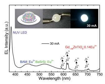
Fig. 9 EL spectrum of the WLED fabricated by the combination of UV LED ( $\lambda \sim 385$  nm), commercial blue-emitting and green-emitting phosphors, and Gd<sub>1.86</sub>ZnTiO<sub>6</sub>:0.14Eu<sup>3+</sup> red-emitting phosphor at the injection current of 30 mA under continuous-wave mode. The schematic illustration of WLED and its photographs before/after the current injection were demonstrated in the inset.
