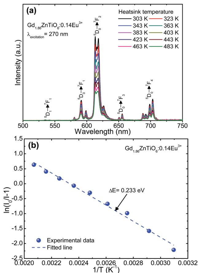
Fig. 6 (a) Temperature-dependent PL emission spectra in the temperature range of 303–483 K with an interval of 20 K and (b) plot of  $\ln(I_0/I - 1)$  versus  $1/T$  of the Gd<sub>1.86</sub>ZnTiO<sub>6</sub>:0.14Eu<sup>3+</sup> phosphor.
