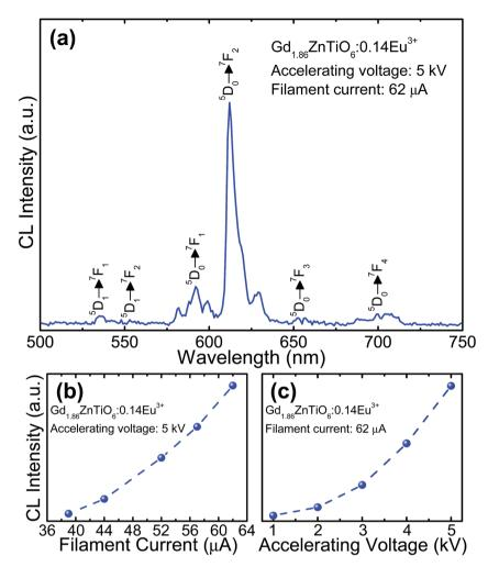
Fig. 10 (a) CL spectrum of the powder under the filament current of 62  $\mu$ A at the accelerating voltage of 5 kV, and CL intensities (b) under different filament currents when the accelerating voltage was fixed at 5 kV and (c) under different accelerating voltages when the filament current was fixed at 62  $\mu$ A.
