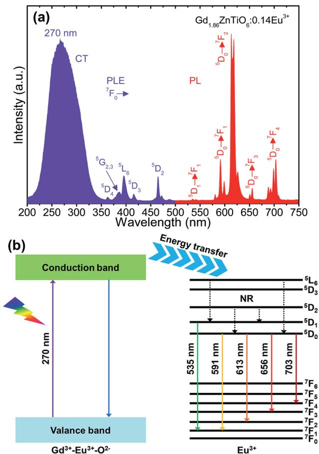
Fig. 4 (a) PLE and PL emission spectra of the  $\text{Gd}_{1.86}\text{ZnTiO}_6:0.14\text{Eu}^{3+}$  phosphor and (b) energy level diagram of the  $\text{Gd}_2\text{ZnTiO}_6$  host material and  $\text{Eu}^{3+}$  ions.
