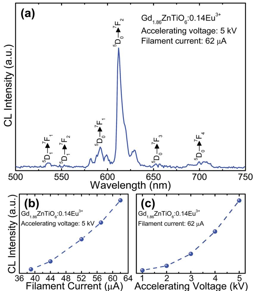
Fig. 10 (a) CL spectrum of the powder under the filament current of 62  $\mu\text{A}$  at the accelerating voltage of 5 kV, and CL intensities (b) under different filament currents when the accelerating voltage was fixed at 5 kV and (c) under different accelerating voltages when the filament current was fixed at 62  $\mu\text{A}$ .
