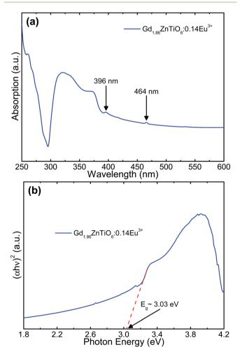
Fig. 7 (a) Absorption spectrum and (b) plot of  $(\alpha h \nu)^2$  versus photon energy of the Gd<sub>1.86</sub>ZnTiO<sub>6</sub>:0.14Eu<sup>3+</sup> phosphor.
