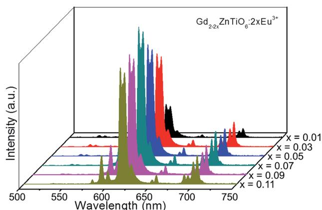
Fig. 5 PL emission spectra of the  $\text{Gd}_{2-2x}\text{ZnTiO}_6:2x\text{Eu}^{3+}$  ( $x = 0.01, 0.03, 0.05, 0.07, 0.09, \text{ and } 0.11$ ) phosphors.
