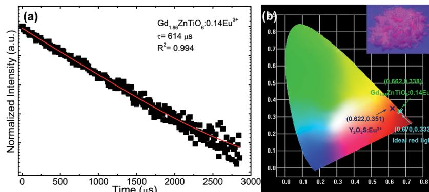
Fig. 8 (a) Luminescence decay curve and (b) CIE chromaticity coordinate of the  $\text{Gd}_{1.86}\text{ZnTiO}_6:0.14\text{Eu}^{3+}$  phosphor. The vivid and intense red color was clearly observed from the powders by naked-eyes as shown in the photograph of (b).
