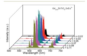
Fig. 5 PL emission spectra of the  $Gd_{2-2x}ZnTiO_6$ : $2xEu^{3+}$  (x=0.01, 0.03, 0.05, 0.07, 0.09, and 0.11) phosphors.
