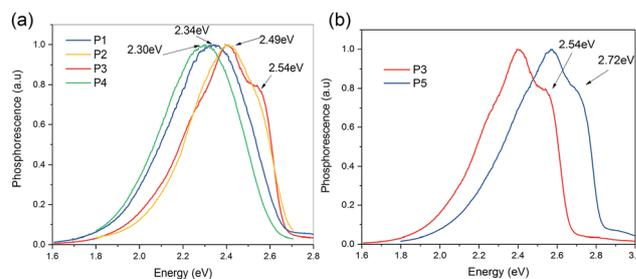
**Fig. 3** (a) The normalized low temperature phosphorescence of **P1**, **P2**, **P3** and **P4** in solutions of dichloromethane. (b) Comparison of the low temperature phosphorescence of **P3** and **P5**.
