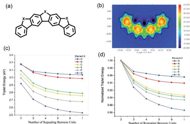
Fig. 5 (a) The general molecular structure of alternating benzene and heterocycle rings where X can be O, N, C, S, P or Si. (b) The ICSS<sub>zz</sub>(1) mapping of four benzene rings separated by pyrrole rings. (c) The triplet energies of extended  $\pi$  systems with different numbers of benzene units separated by different heterocycles. (d) The normalized triplet energies with different numbers of repeating benzene units.
