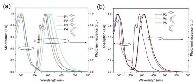
**Fig. 2** (a) The normalized absorption and photoluminescence of **P1**, **P2**, **P3** and **P4** in solutions of dichloromethane. (b) Comparison of the absorption and photoluminescence of **P3**, **P4** and **P5**.
