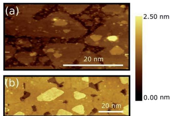
Fig. 1 (a) STM topographic images of the MoS<sub>2</sub> ML ( $V_{\text{tip}}$ : 1.0 V,  $I_{\text{Tunnel}}$ : 100 pA) (b) STM topographic images of the MoS<sub>2</sub> BL ( $V_{\text{tip}}$ : 1.0 V,  $I_{\text{Tunnel}}$ : 50 pA). STM images were acquired at 77 K of sample temperature. The colour scale indicates the relative height variation from HOPG (darker area) to top MoS<sub>2</sub> layers (brighter areas).
