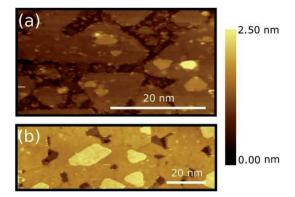
Fig. 1 (a) STM topographic images of the  $MoS_2$  ML ( $V_{tip}$ : 1.0 V,  $I_{Tunnel}$ : 100 pA) (b) STM topographic images of the MoS<sub>2</sub> BL ( $V_{\rm tip}$ : 1.0 V,  $I_{\rm Tunnel}$ : 50 pA). STM images were acquired at 77 K of sample temperature. The colour scale indicates the relative height variation from HOPG (darker area) to top MoS<sub>2</sub> layers (brighter areas).
